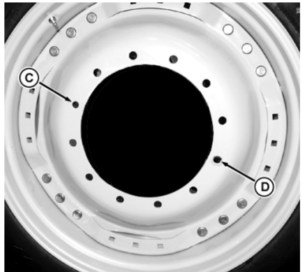
A—Disk-to-Rim Tight Fit Hole C—Disk-to-Hub Tight Fit Hole B—Disk-to-Rim Slot Fit Hole D—Disk-to-Hub Slot Fit Hole
