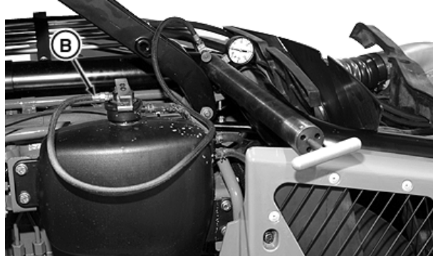
Attach Radiator Tester
