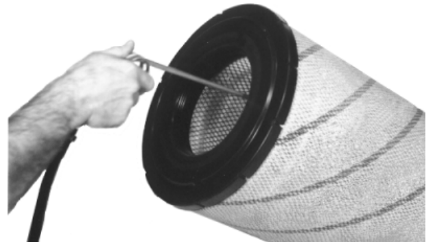
Clean And Inspect Primary Filter
