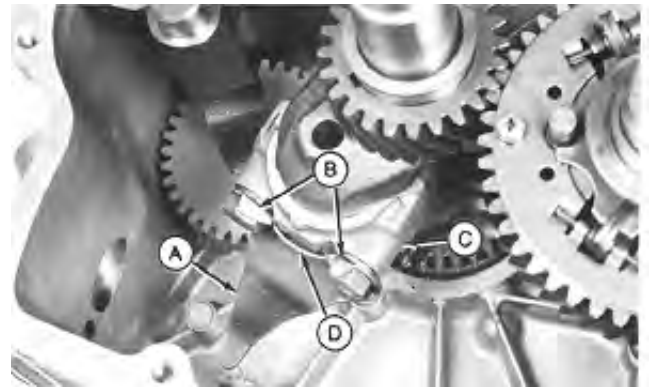
A—Oil Splasher B—Locking Tabs C—Connecting Rod Cap D—Lock Plate
