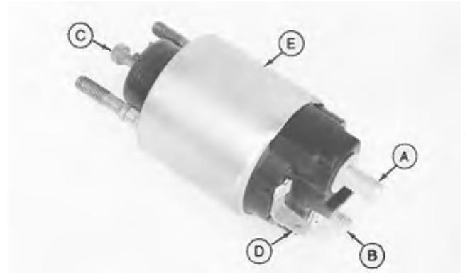
A—Terminal B—Terminal C—Switch Arm D—Tang E—Solenoid Body
