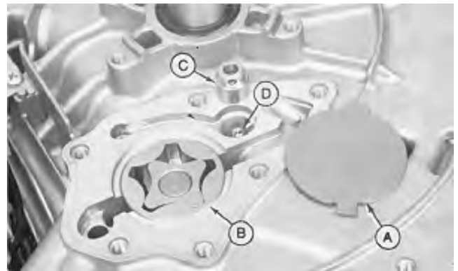
A—Plate B—Oil Pump Assembly C—Relief Valve D—Relief Spring and Ball
