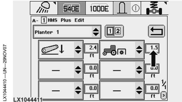
Step 4: Enter distance the tractor moves until the next function is activated
