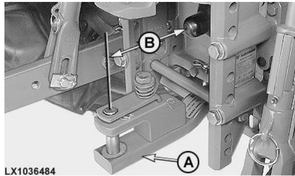
If PTO splines are not aligned with the grooves in the u.j. shaft, keep the engine shut off and select “N” cell at the CommandCenter. Then turn the PTO shaft manually to the correct position.
