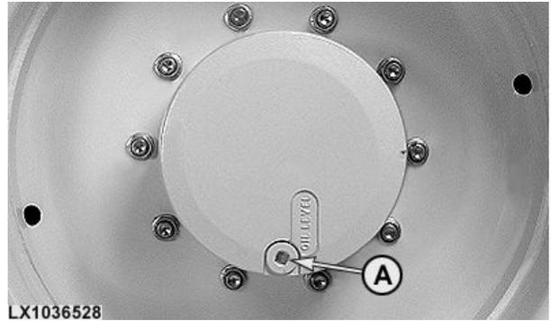
3. Reinstall drain screw and tighten to 120 Nm (90 lb-ft).
