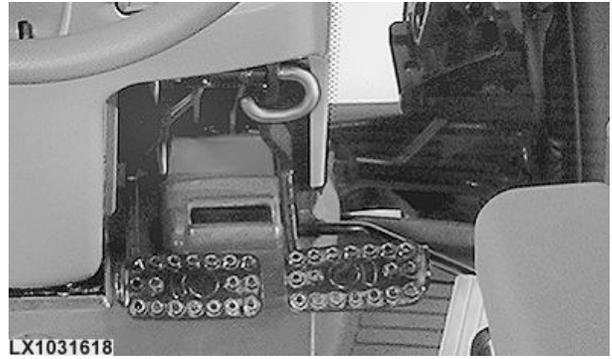
*Also use the brake pedals when turning on a downhill slope, as this will make the tractor change direction faster.*
