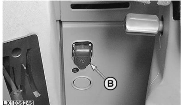
3-terminal socket in rear cab wall
