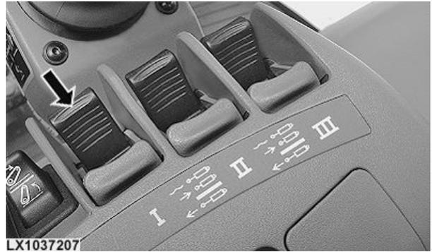
To re-activate the automatic shut-off, cycle the SCV control lever back from beyond the point of resistance and then past the point of resistance again.
