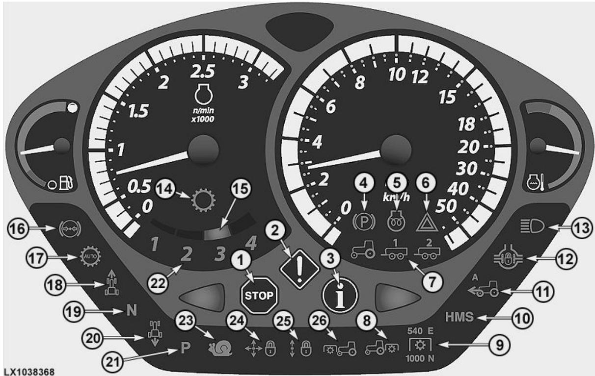
1-The red STOP light flashes when a serious malfunction occurs. Switch off the engine IMMEDIATELY and determine the cause (review the error message in the CommandCenter).
