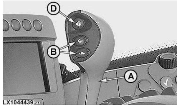
Range-shift lever and buttons (with hand clutch)
