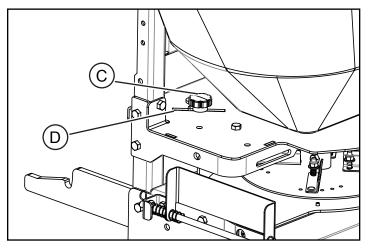
Position the knob in the end of the slot at position (D) for maximum material output.
