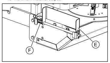
3. The barrier shield (E) comes installed on the left side of the fertilizer spreader. To raise or lower the shield, push it against the spring (F) and rotate.
