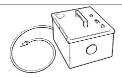
**12V Mobile Oven** - 1 cartridge capacity - required to pre-heat adhesive prior to use. It is fitted with a male plug (703/23201) which fits into a female socket (715/04300).
