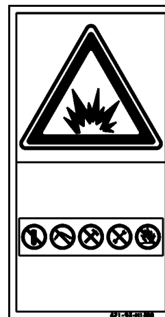
10 High pressure warning (421-93-H1300)
