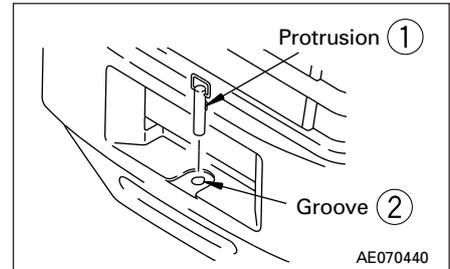
2. To prevent the towing pin from turning, bend the towing pin handle down and set it in position.
