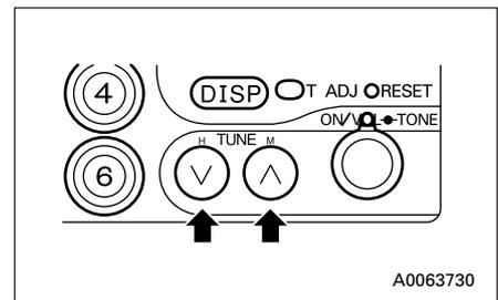
If the reception is weak, and stations are not found, adjust the frequency manually to select the desired station.
