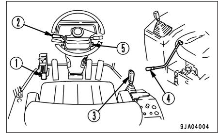
1. Check that parking brake pedal ① is at the LOCK position.
