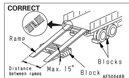
2. Determine the direction of the ramp, then slowly load or unload the machine.
