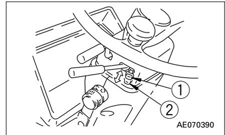
**4. SAFETY LOCK LEVER (for work equipment control lever)**
