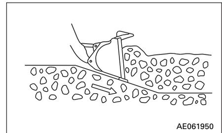
3. Operate the work equipment control lever slightly up and down to reduce the resistance when driving the machine forward.
