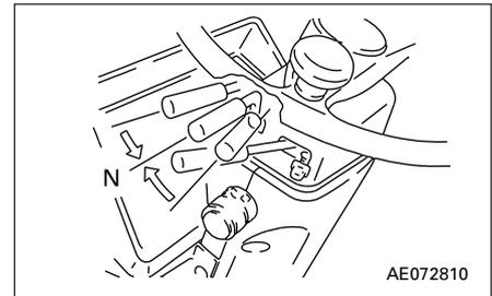
3. Lower the bucket to the ground, then check that work equipment control lever ③ is locked by safety lock lever ④.
