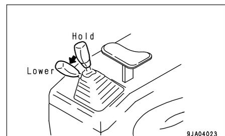
5. Lock work equipment control lever ⑤ with safety lock lever ⑥.
