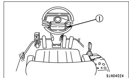
2. Turn the key in starting switch ① to the OFF position and stop the engine.
