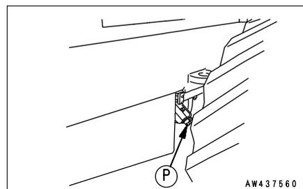
**CHECK AND REFILL OF OIL IN BRAKE OIL TANK**
