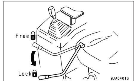
This is used to lock the work equipment levers.
