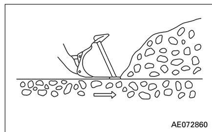
2. After the bucket has fully penetrated into the soil, place the work equipment control lever in raise position while moving the machine forward. Move the work equipment control lever to tilt position from time to time until the bucket is filled with soil.
