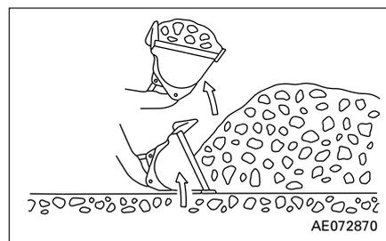
3. When it is difficult for the bucket to penetrate into the piled soil, move the work equipment control lever left and right to move the bucket teeth up and down.
