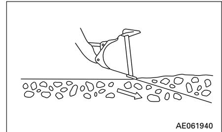
2. Drive the machine forward and operate the work equipment control lever forward to cut a thin layer of the surface each time when excavating the soil.
