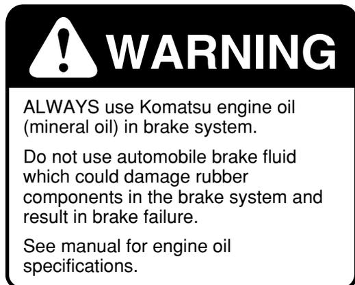
A black and white warning sign with a white background. At the top, a black triangle with a white exclamation mark is followed by the word "WARNING" in bold black letters. Below this, the text reads: "ALWAYS use Komatsu engine oil (mineral oil) in brake system. Do not use automobile brake fluid which could damage rubber components in the brake system and result in brake failure. See manual for engine oil specifications."
