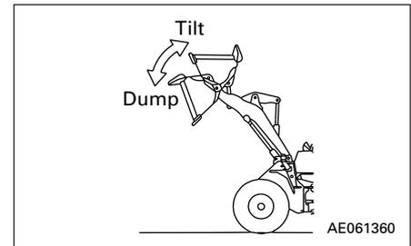
When the work equipment control lever is pulled further from the TILT position, the lever is stopped in this position until the bucket reaches the preset position of the positioner, and the lever is returned to the HOLD position.
