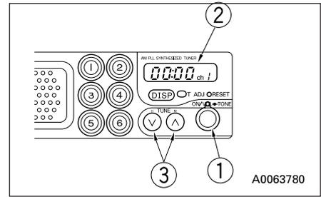
After programming the button, press the preset button and release it within approx. 2 sec. The station programmed to that button will be selected for reception.
