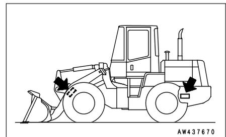
5. When the machine leaves the ground, stop for a moment and wait for the machine to stabilize, then continue the lifting operation slowly.
