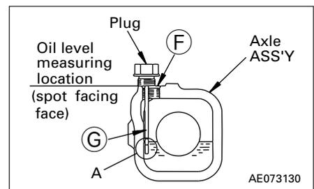
5. If the oil level is above the upper line, drain off the excess oil through drain plug ⑤ and check the oil level again.
