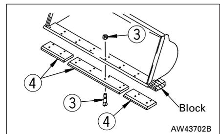
If both sides of the cutting edge are worn, replace with a new part.
