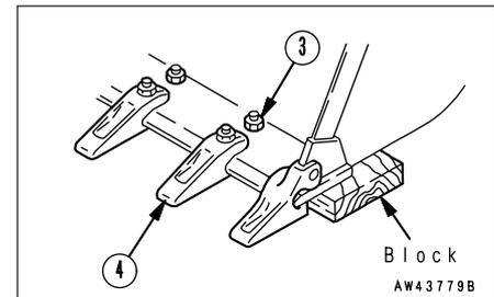
If the mounting surface is worn, correct the mounting surface before installing the teeth.
