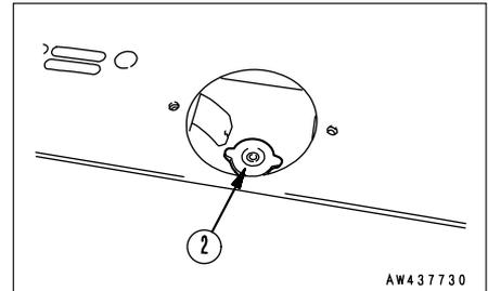
3. Prepare a container to catch the coolant, then open drain valve ③ at the radiator left lower portion to drain the coolant.
