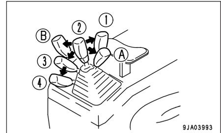
When the work equipment control lever is pulled further from the RAISE position, the lever is stopped in this position until the lift arm reaches the preset position of the kick-out, and the lever is returned to the HOLD position.
