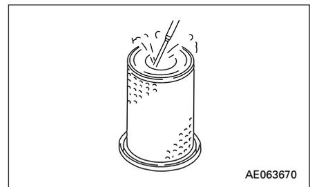
3. Direct dry compressed air (less than 700 kPa (7 kgf/cm<sup>2</sup>, 100 psi)), to the element from inside along its folds, then direct it from outside along its folds and again from inside.
