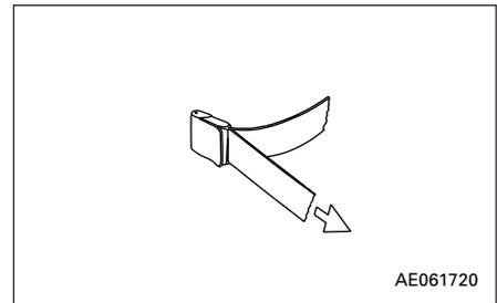
To make belt longer: Set the belt holding the buckle or tongue end at right angles to the buckle or tongue, and pull.
