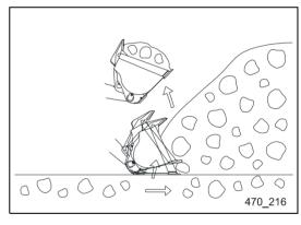
8. If there is too much material inside the bucket, you must briefly tip it in, dump it and lower it in order to reduce the load and to prevent that you lose the load during the transport.
