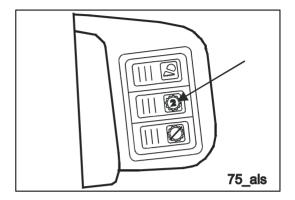
2. Press the ALS-Electronics switch. The green control lamp in the switch lights up.
