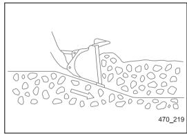
Move the multi-function lever of the boom slightly up and down to reduce the resistance during driving forward.
