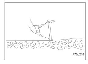
4. While driving forward, move slightly the multi-function lever of the boom in order to remove only a thin layer of the surface of the soil to be removed.
