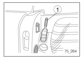
6. Set the drive direction switch to the desired direction setting.
