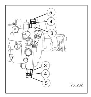
After towing another machine loosen the counter-nut (4) and the threaded stud (5) by turning it anti-clockwise until it reaches the limit stop. Hold the valve (3) in position using a wrench an retighten firmly the counter-nut (4). Perform these operations on both valves.
