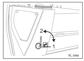
Release the parking brake. Press the celebration adjustment knob to this at the parking brake lever. Press down the locking button of the parking brake lever. Then, release the locking button. The parking brake warning light goes out.
