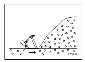
5. Press down the accelerator pedal and drive the bucket into the material to be removed. In order to remove the material, it is required that you align horizontally the cutting edge of the bucket while driving into the material. When you are loading rock debris, it is necessary to lower the bucket slightly.
