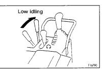
2. Place steering and directional lever 2 in the N (neutral) position.
