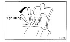
3. Increae engine speed by fuel control lever ①.
