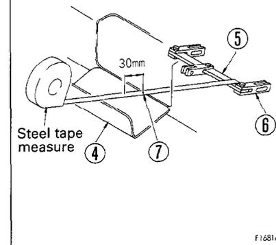
6. The travel at the tip of the pedal should be 110 mm when the brake pedal is depressed fully.
