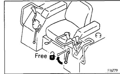
6. Set gear shift lever ③ to a desired position, set steering and directional lever ④ to the forward or reverse position.
