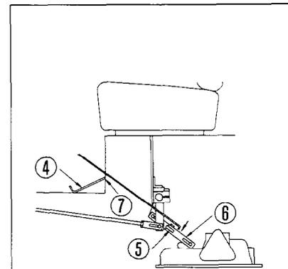
5. Read the movement of the steel tape (lever ⑤) while the brake pedal is depressed fully.
