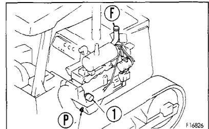
8. After replacing the filter cartridge, add engine oil through oil filler
