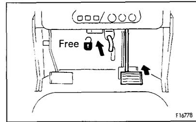
5. Set safety lever ③ for the steering and directional lever to the FREE position.
