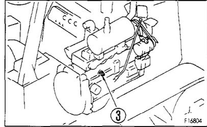
12. To remove the air in the cooling water, run for five minutes at low idling, then for another five minutes at high idling.
