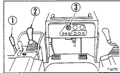
1. Pull fuel control lever ① to the center position between LOW IDLING and HIGH IDLING and run the engine at medium speed for about 5 minutes with no load.
