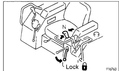
3. Check that the blade is lowered on the ground and the blade control lever is locked with safety lever ④.
