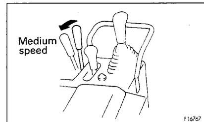
2. When starting in cold weather, operate the steering and directional lever ② as follows. Move steering and directional lever ② to the N position, move the lever fully in left direction ④ and hold it for 5 seconds, then move the lever fully in right direction ⑤ and hold it for 5 seconds. Repeat this operation in each direction in turn for 5 minutes with engine running under no load.
