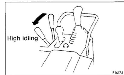
2. Set safety lever ⑥ for blade control lever ⑦ to the FREE position.
