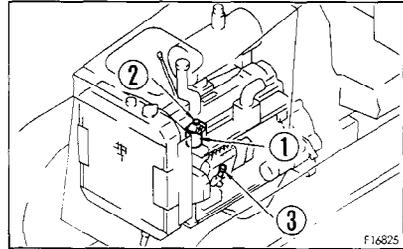
7. Tighten up air bleeding plug ②. Push in the knob of feed pump ③ and tighten it.
