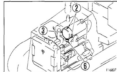
3. Direct dry compressed air (less than 7 kg/cm<sup>2</sup>) to the element from inside along its folds, then direct it from outside along its folds and again from inside.
