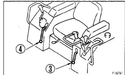
1. Check that the brake pedal is locked with brake lock lever ①.
