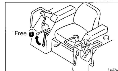
3. Put blade control lever ⑦ in the RAISE position to raise the blade 400 to 500 mm off the ground.
