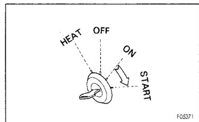
3. When the engine starts, release the key in starting switch ②. The key will return automatically to the ON position.
