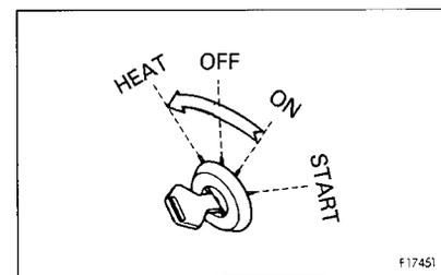
If the preheating time is too long or too short, the engine will not start easily. Observe the correct preheating time.
