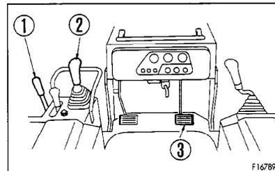
1. Lower engine speed by operating fuel control lever ①.
