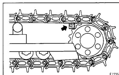
2. Measure pitch length of 4 links in stretched portion at more than 2 links away from master pin. Of length obtained, 1/4 is the link pitch.
