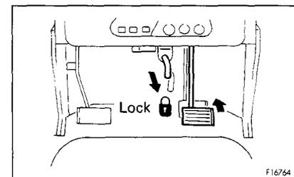
5. Lock steering and directional lever ② with safety lever ⑤.
