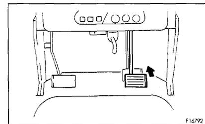
4. Pull brake lock lever ④ and depress brake pedal ③ strongly to apply the lock securely.
