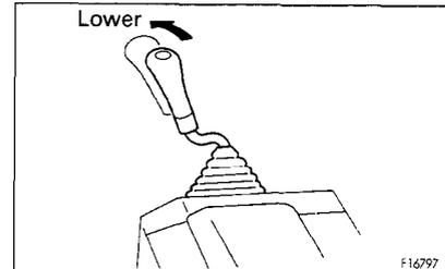
7. Lock blade control lever ⑥ with safety lever ⑦.
