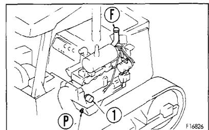
8. After replacing the filter cartridge, add engine oil through oil filler
