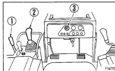
1. Pull fuel control lever ① to the center position between LOW IDLING and HIGH IDLING and run the engine at medium speed for about 5 minutes with no load.
