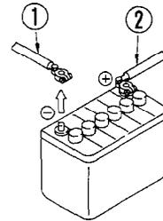
When installing, install the positive  $\oplus$  terminal first.
