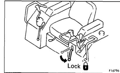
6. Put blade control lever ⑥ in the LOWER position to lower the blade to the ground while keeping it horizontal.
