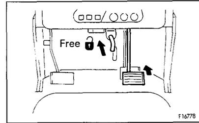
5. Set safety lever ③ for the steering and directional lever to the FREE position.
