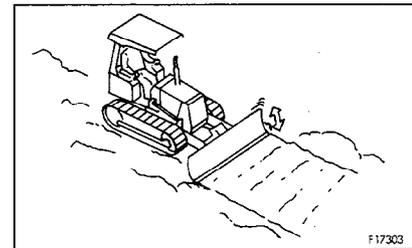
The D31PL, PLL can be used for leveling of fields where there are no rocks when the ground is too soft for standard swamp bulldozers to operate.
