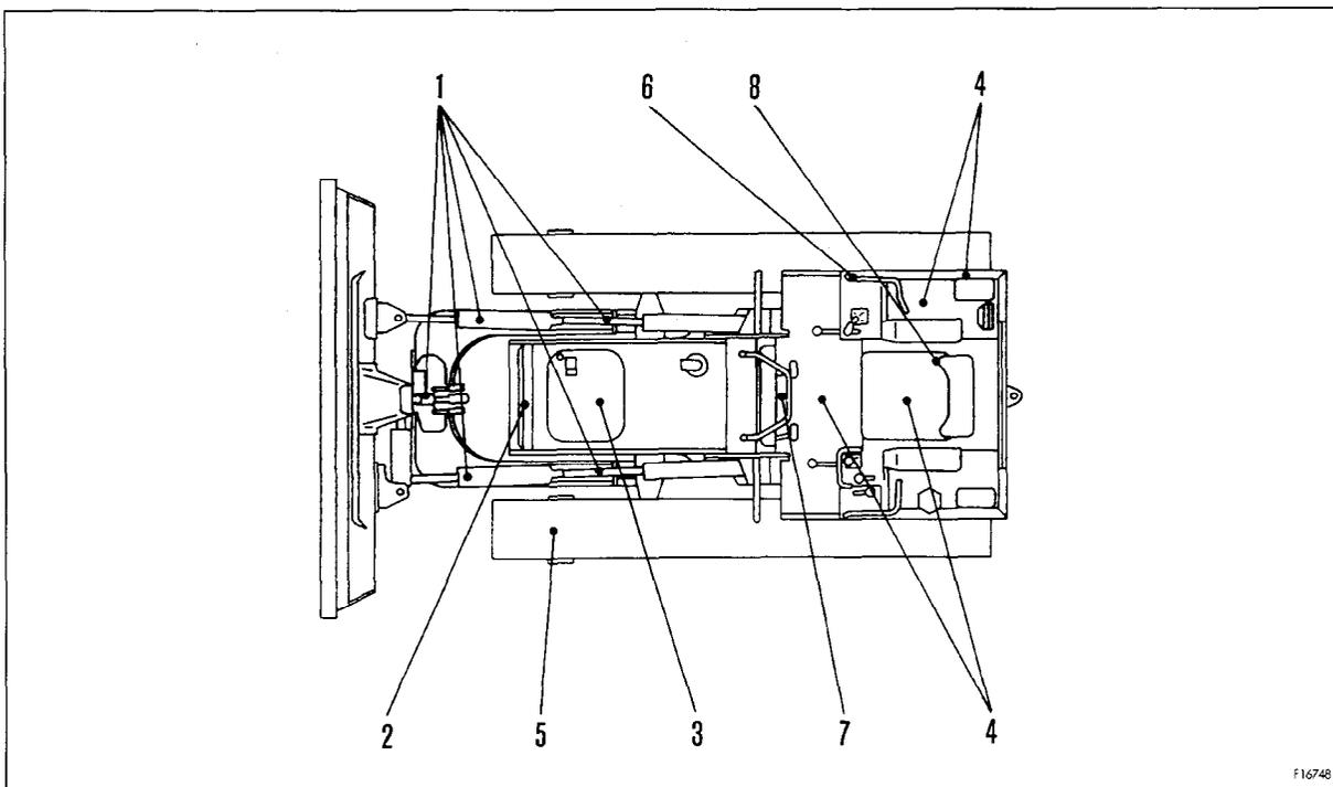
1. Check for damage, wear, play in work equipment, cylinders, linkage, hoses
