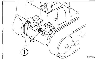
2. Tighten adjustment nuts ②, ③ to torque of 4 kgm until the lining contacts the drum. Then, turn adjustment nuts ②, ③ in reverse directions for 2.5 rotations.
