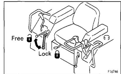
This is the locking device of blade control lever. Lower the lever to apply the lock.
