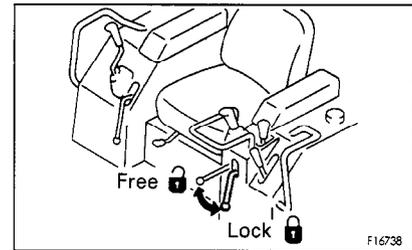
This locks the steering and directional lever. Move the steering and directional lever to the N (neutral) position and lower the lever to apply the lock.
