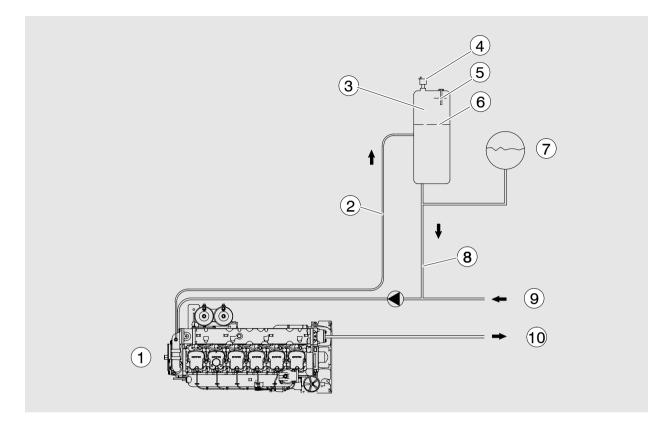
Diagram of cooling system with diaphragm expansion vessel
