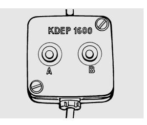
Slowly turn the engine further until lamp (B) comes on too. The injection pump is now at start of delivery.
