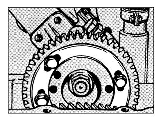
Remove cover above the injection pump drive gear. Losen the fixing bolts joining the drive gear to the injection pump hub.
