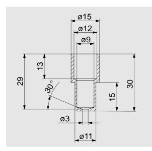
The receptacle is to be made of aluminium or steel in accordance with the drawing (figure).
