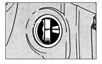
Then rotate engine so that mark on pointer fitted to injection pump coincides with mark on drive gear.
