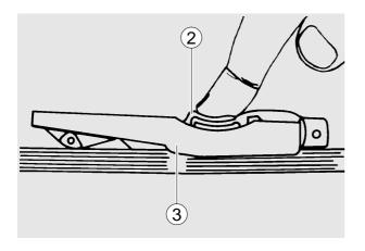
• Slowly depress pad ③ until the spring can be heard to disengage. This will cause the indicator to move upwards
