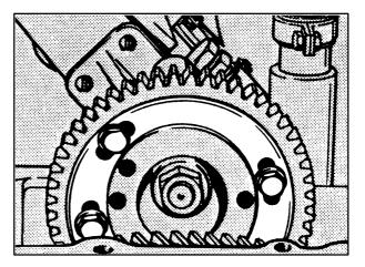
Remove cover above the injection pump drive gear
