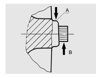
A = Point of support for dial gauge tipB = Measuring capacity
