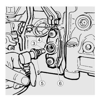
Connect up power supply of light signal transmitter (red terminal = +). Turn engine by hand so that piston in cylinder no. 1 in the compression stroke comes close to the start of delivery.
