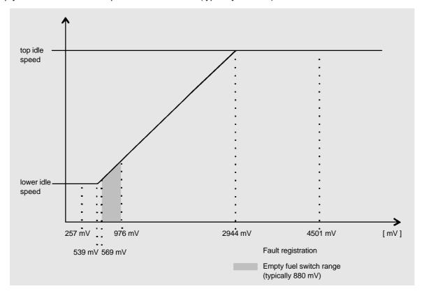
Exceptionally, the voltage "u" is produced electronically as drive position selection, or the setpoint selection (drive position selection) takes place via the CAN bus.
