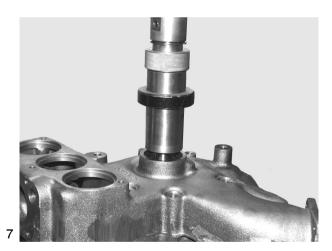
Fig. 8 Press V-belt pulley flush on to bearing shaft.
