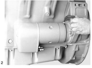
Check flywheel gear ring for wear and damage.
