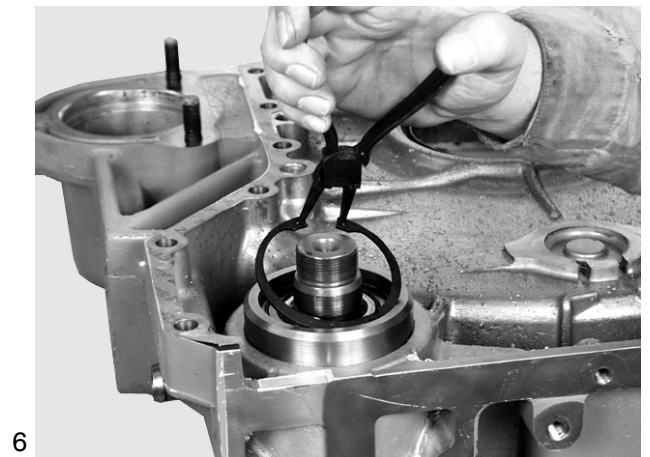
Fig. 6 Unclip circlip. Press power take-off for raw-water pump out of timing case.
