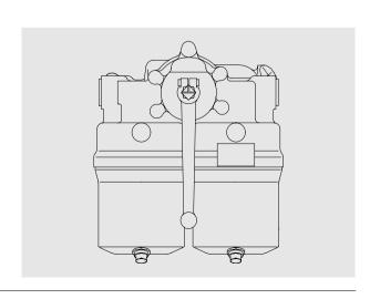
During continuous operation position the selector lever that both filter halves are in operation.
