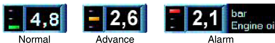
Figure: Example of a display with alarms
