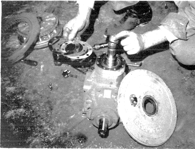
Figure 10. Sleeve & Shims, Bearing Preload Adjustment
