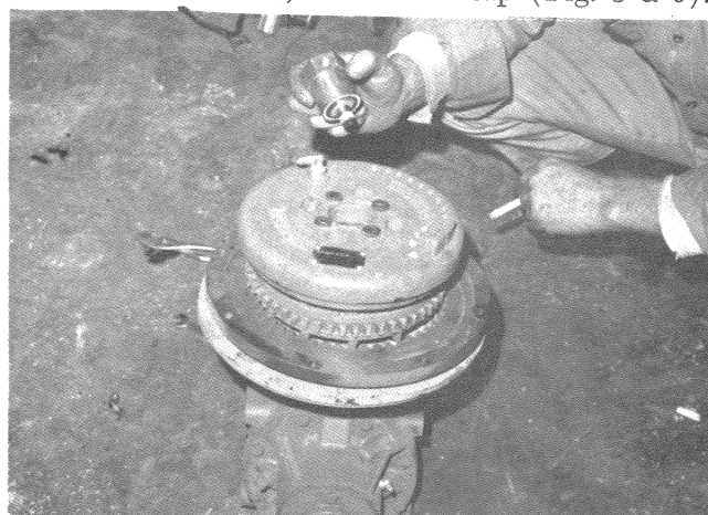
Figure 6. Clutch End-cap, removed
