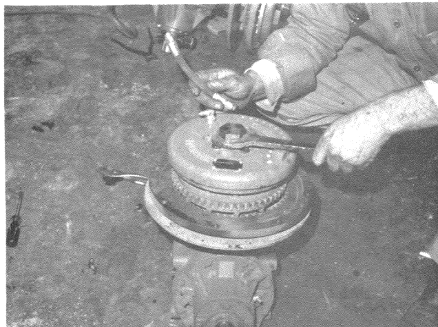
Figure 5. Clutch Air line and End-Cap
