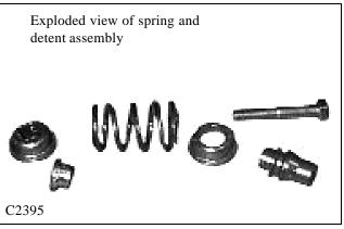
25 To remove the detent mechanism and spring from the spool, place an allen wrench or screwdriver blade through the spool eyelet to hold the spool from turning while removing the spring and detent mechanism. (fig. C2394).
