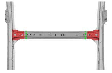
Use a tram gauge to measure the distance between the center of the trim hole on the underside of each Rear Header Connector and the center of the trim hole on the underside of the opposite Front Header Connector (trim holes highlighted in red).
