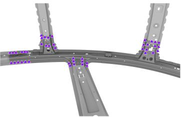
Clean all the mating surfaces of the new component or components and the vehicle with isopropyl alcohol (IPA).
