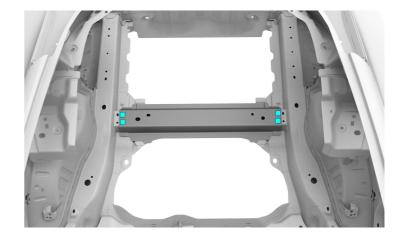
Use a heat gun to heat the adhesive joints, and then use a hammer and chisel to remove the remaining pieces of the original component.
