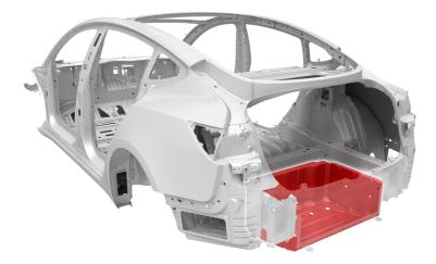
Remove the Rear Motor Cover Floor.
