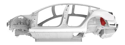
Install the Trunk Floor Assembly (Complete).
