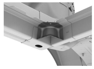
Use an SPR removal tool or a drill with a high-strength steel bit to remove the factory self-piercing rivets. Use a belt sander for any factory self-piercing rivets that cannot be removed with an SPR removal tool or a drill.
