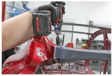
Create holes for flow form rivets.
