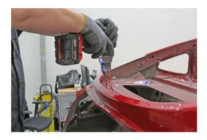
Use a belt sander to grind down enough of the heads of the factory self-piercing rivets shown to remove the original component.
