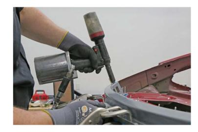
Install the flow form rivets.
