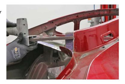
Grind down any remaining pieces of the factory self-piercing rivets so that the Parcel Shelf is flush.
