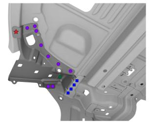
Install all structural, countersunk, and Flow Form rivets.
