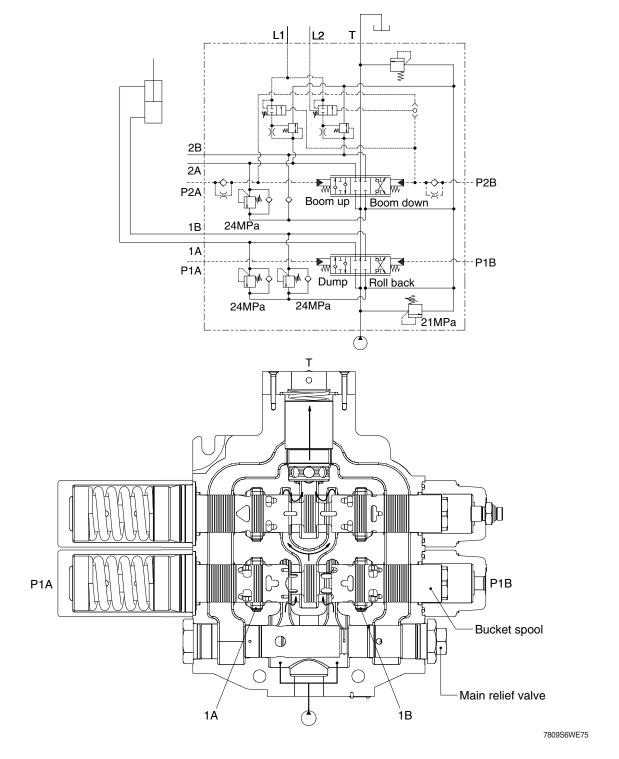
If the remote control value is not operated, the oil supplied from the pump port passage through the neutral passage to the low pressure passage at the outlet section, and then return to the tank port.
