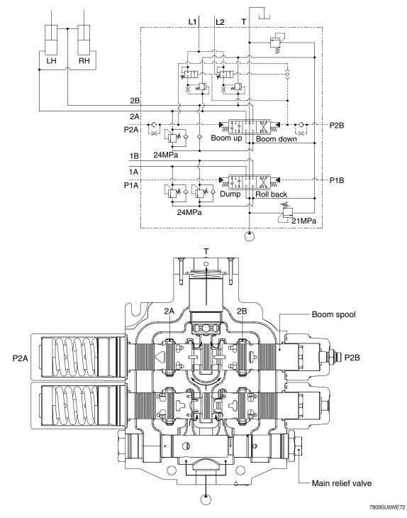
If the remote control valve is not operated, the oil supplied from the pump port passes through the neutral passage to the low pressure passage at the outlet section, and then returns to the tank port.
