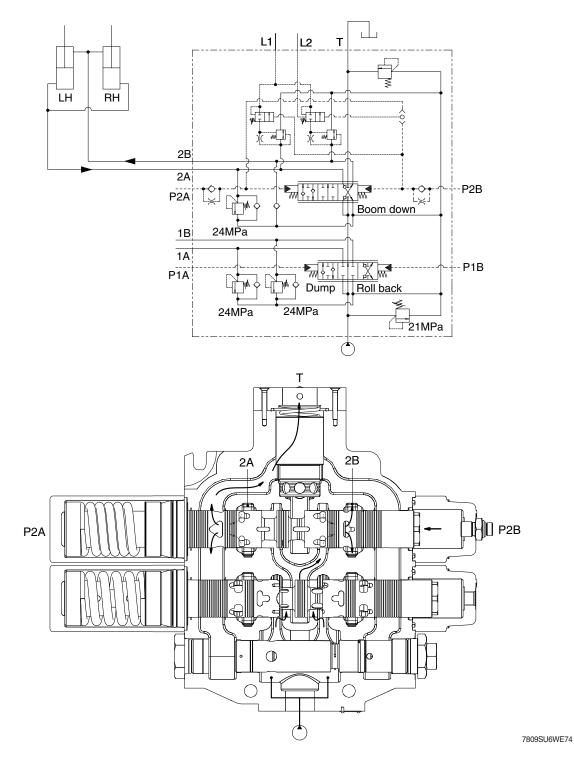
When the pilot pressure from remote control valve is supplied to the pilot port (P3B), the spool moves to the left and the neutral passage is closed.
