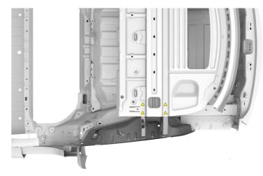
Use a drill with a 6.7 mm bit to drill completely through the spot welds shown.
