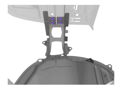
Put the new component into position and align it to the frame bench jig points.
