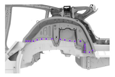
Insert the structural bulb rivets.
