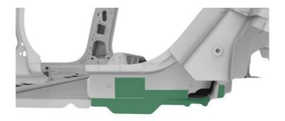
Mark the installation spot weld locations on the new component and on the vehicle.
