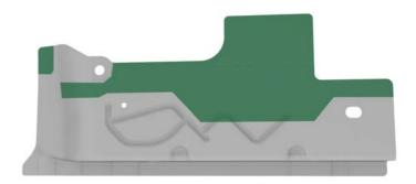
Mark the bond path areas on the new component and the vehicle. These areas will be prepared for bonding in the next step.
