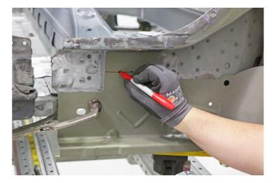
Use a drill with a 6.7 mm (17/64 in) bit to drill holes for structural rivets.
