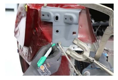
Use a drill with a 4.8 mm (3/16 in) bit to drill holes for structural rivets.
