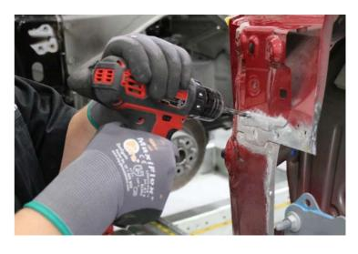
Use an SPR removal tool or a drill with a high-strength steel bit to remove the factory self-piercing rivet.
