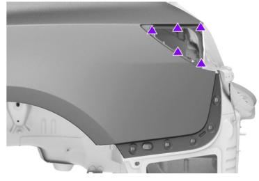
Mark the locations for plug welds on the deck lid area of the new component.
