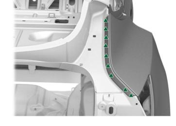
Right-hand component only: Plug weld the steel areas.
