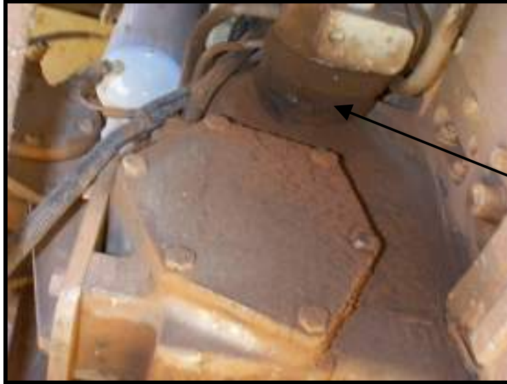
Fig. 30 Low-pressure fuel leak at weep hole.
