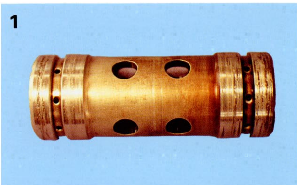
Journal bearing scuffed and worn excessively due to lack of lubricating oil.
