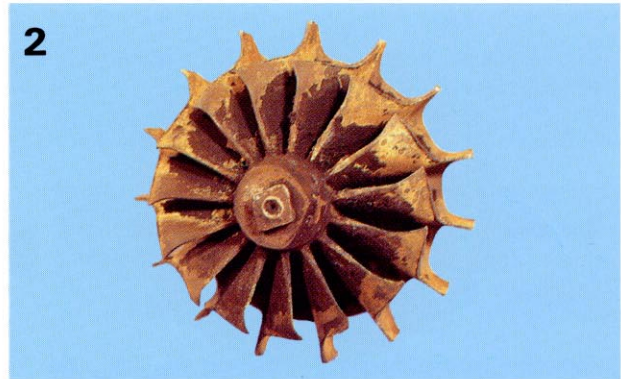
Turbine impeller deformed by foreign matter.
