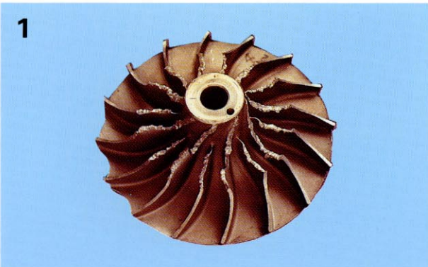
Blower impeller damaged with foreign matter like stones, nuts, washers, etc.
