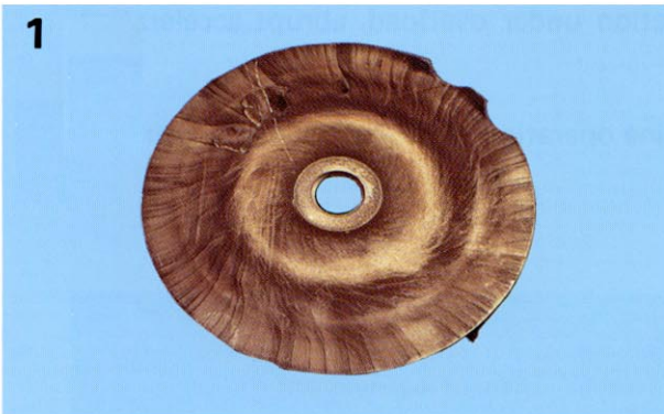
Oil adhering to back face of blower impeller.
