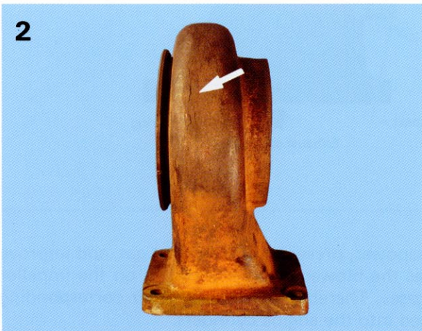
Turbine housing with heat cracks.
