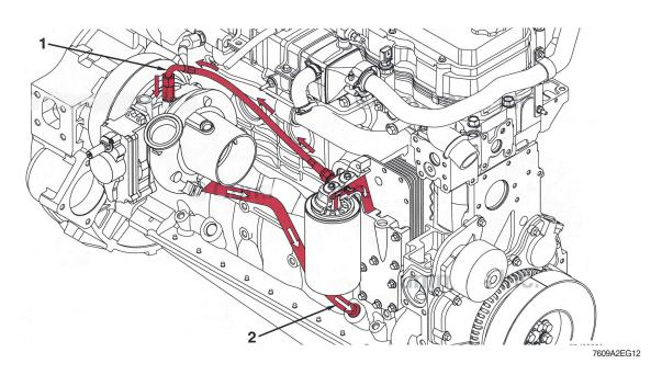
1 Turbocharger lubricating oil supply
