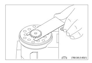
(25) Grease the two O-rings with mineral oil approx. viscosity 500 cSt at 20°C and place them in the two grooves in the gear rim. Fit the gearwheel and rim on the cardan shaft.
