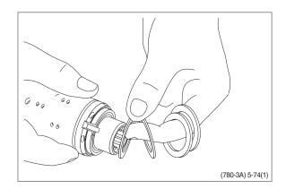
(10) Press out the cross pin. Use the special screw from the end cover.
