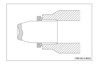
(15) Guide the assembly tool right to the bottom.
