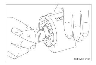
(18) The spool set will push out the assembly tool guide. The O-ring are now in position.
