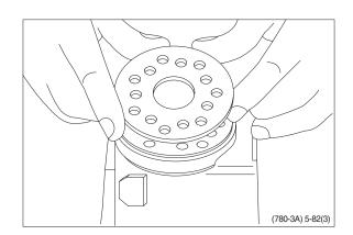
(23) Guide the cardan shaft down into the bore so that the slot is parallel with the connection flange.
