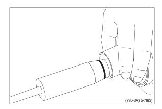
(12) Press and turn the O-ring into position in the housing.
