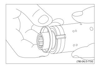
(7) Fit the cross pin into the spool / sleeve.
