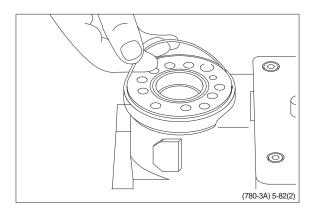
(22) Place the distributor plate so that the channel holes match the holes in the housing.
