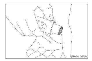
(13) Remove dust seal and O-ring.
