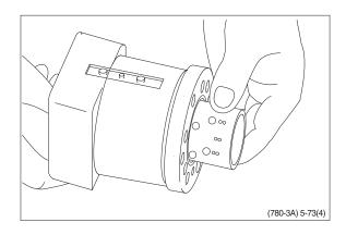
(9) Take ring, bearing races and needle bearing from sleeve and spool. The outer (thin) bearing race can sometimes "stick" in the housing, therefore check that it has come out.
