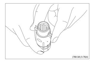
(3) Assemble the spool/sleeve and make sure the marks on spool and sleeve are opposite each other (see drawing page 5-36).
