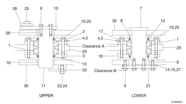
Assemble the center pivot group by reversing the order of disassembly while paying close attention to the following.
