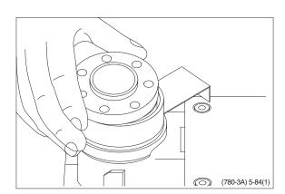
(29) Fit the special screw with washer and place it in the hole shown.
