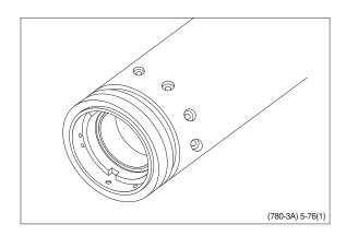
(4) Press the springs together and push the neutral position springs into place in the sleeve.
