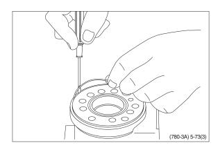
(8) Take care to keep the cross pin in the sleeve and spool horizontal. The pin can be seen through the open end of the spool. Press the spool inwards and the sleeve, ring, bearing races and needle bearing will be pushed out of the housing together.
