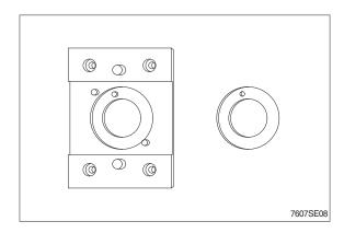
(2) Assembly tool for O-ring and kin-ring.
