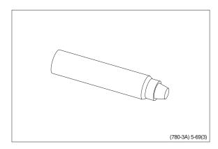
(4) Assembly tool for cardan shaft.
