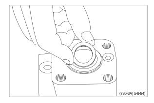
(32) Fit the dust seal ring in the housing using special tool and a plastic hammer.
