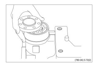
(3) Lift the gearwheel set (with spacer if fitted) off the unit. Take out the two O-rings.
