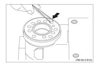
(20) Screw the threaded bush lightly into the check valve bore. The top of the bush must lie just below the surface of the housing.
