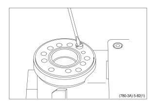
(21) Grease the O-ring with mineral oil approx. viscosity 500 cSt at 20°C.
