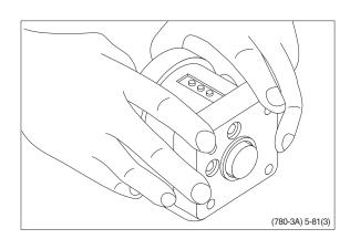
(19) Turn the steering unit until the bore is vertical again. Put the check valve ball into the hole indicated by the arrow.
