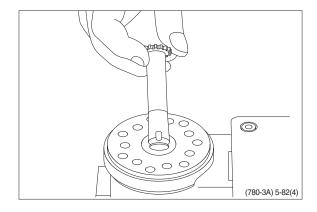
(24) Place the cardan shaft as shown - so that it is held in position by the mounting fork.
