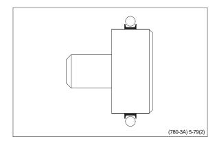
(11) Hold the outer part of the assembly tool in the bottom of the steering unit housing and guide the inner part of the tool right to the bottom.
