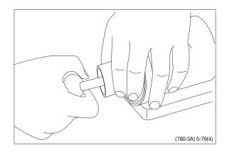
(13) Draw the inner and outer parts of the assembly tool out of the steering unit bore, leaving the guide from the inner part in the bore.
