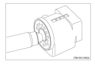
(16) Press and turn the lip seal into place in the housing.
