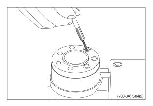
(30) Fit the six screws with washers and insert them. Cross-tighten all the screws and the rolled pin.
