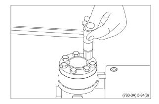
(31) Place the dust seal ring in the housing.
