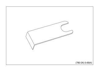
(5) Assembly tool for dust seal.
