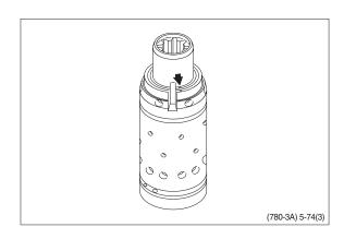
(11) Carefully press the spool out of the sleeve.
