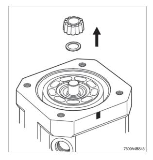
(7) Remove the rotary group in a horizontal position.
