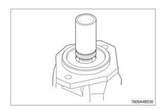
(6) Assemble the circlip.
