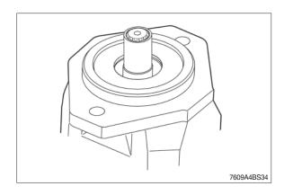
(5) Use a suitable pipe to mount the shaft seal, but don't push it too deep. If the shaft ring touches the bearing ring you will damage the seal ring.
