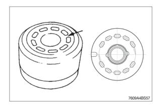
(5) Mounting surface - control plate undamaged.
