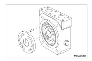
(5) Remove bearing outer ring with withdrawal tool.
