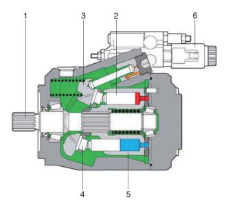
The pump is a variable displacement piston pump. This pump has a maximum delivery pressure of 250 kgf/cm<sup>2</sup>. The axial piston type pump is used to supply oil flow to the cut off valve. The oil is pressurized by the movement of rotary group in the pump.
