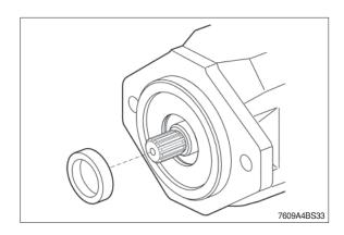
(4) Use installation tool or plastic strip for assembling seal.
