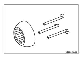
(4) Cylinder sliding surface free of grooves, no wear, no embedded foreign particles. That there are no scratches on the control plate. (Only replace them as a set).
