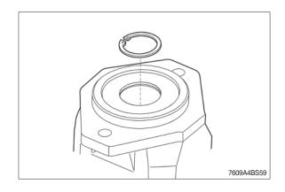
(2) Assemble shaft seal and shim against circlip.
