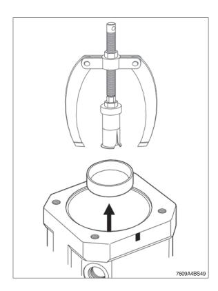
(13) Disassemble circlip and shaft seal.
