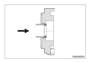
(14) Remove shaft seal and shim.
