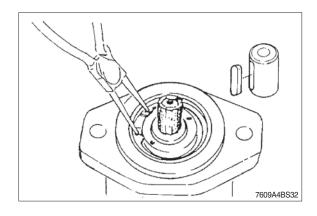
(3) Change the shaft seal and check its sliding surface (drive shaft) and housing, grease the sealing ring.
