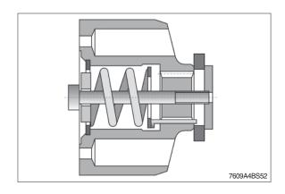
(16) Remove circlip.
