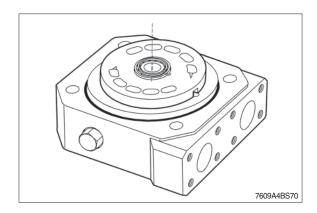
(12) Fit the port plate and fix it with the bolts crosswise.
