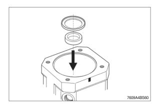
(3) Assembly of the shaft seal (1) against the safety ring (2) back up the shim (3) down to the seal ring.
