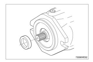
(2) Assembling of the sealing ring carefully down to the stop ring.
