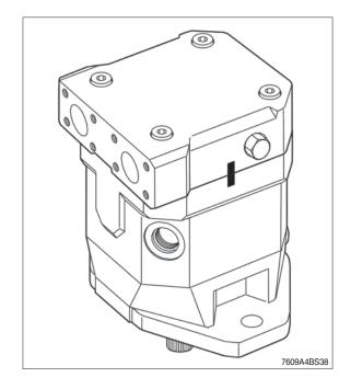
(2) Remove the port plate fixing bolts crosswise.
