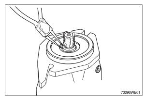
\* Change the shaft seal and check its sliding surface (drive shaft) and housing, grease the sealing ring.
