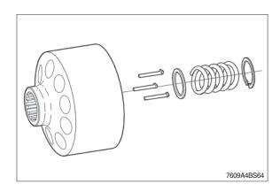
(7) Pre-tension the spring using a suitable device.
