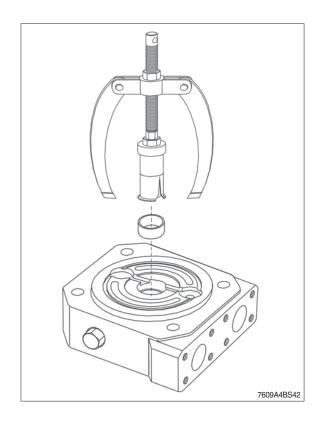
(6) Disassemble the taper roller bearing (near by port plate).
