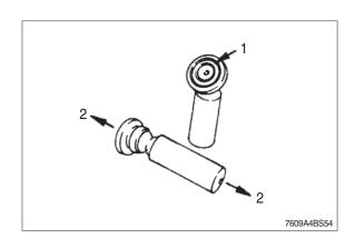
(2) Check cylinder bores (1) and splines (2).
