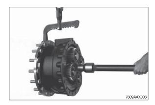
⑥ Fix output to assembly truck.
