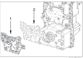
⑤ Pull converter safety valve (1) out of housing hole.
