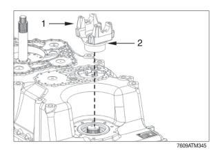
③ Insert O-ring 48×4 into the space between output flange and shaft.
