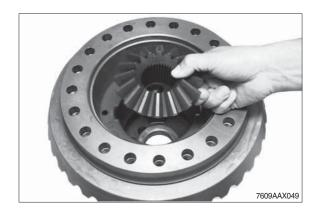
② Press crown wheel from the differential carrier.
