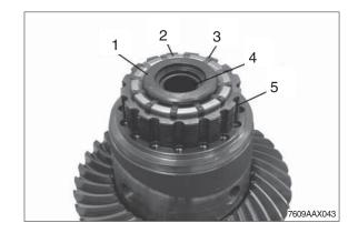
⑥ Preload differential by means of the press, loosen locking screws and housing cover.
