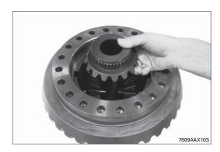
Insert the second pressure ring into the differential housing.
