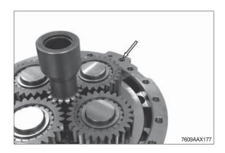
③ Grease O-ring (see arrow) and install it to the axle housing.
