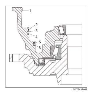
⑥ Flush - mount slotted pins (for installation position refer to arrow) into the piston if not disassembled, adjust adequately (flush-fitting).
