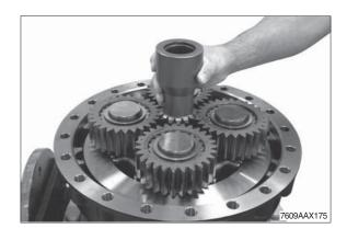
③ Fix determined shim (s) e.g. s = 1.60 mm with grease into the sun gear shaft.
