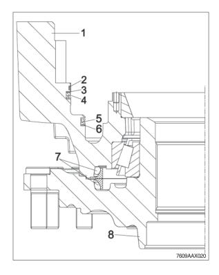
(9) Lift the brake housing from the output shaft by means of the lifting device.
