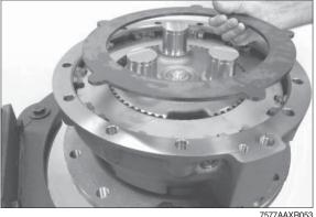
\* Make leakage test on brake hydraulics.
