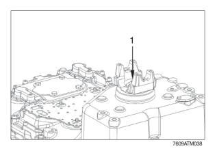
② Pull off output flange (1) and remove shaft seal (2).
