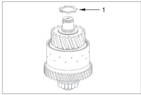
④ Remove axial bearing assy (1).
