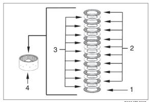
9 Mount end plate (1) and fix disk package by means of snap ring (2) (e.g. thickness = 2.65 mm / recommended value).
