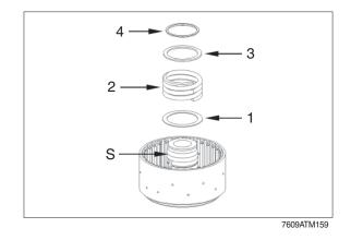
Preload compression spring by means of assembly aid (S1) and pressure piece (S2), until L-ring has engaged into the annular groove.
