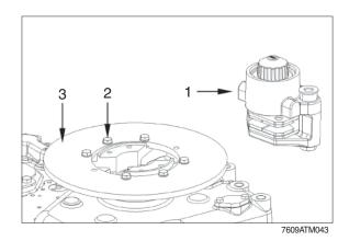
⑤ Loosen hexagon screws (1), remove washer and O-ring.
