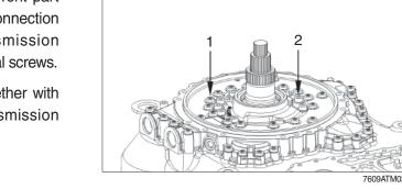
3 Separate oil pressure pump (1) from oil feed housing (2).
