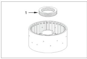
(3) Lift piston (1) by means of compressed air out of the cylinder bore and remove it.
