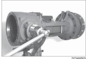
④ Remove disc and pull-off flange.
