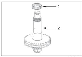
$\ensuremath{\otimes}$  Turn shaft (2) by 180° and snap out piston ring (1).
