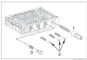
**(3) Lock-up clutch solenoid valve** (5-speed transmission)
