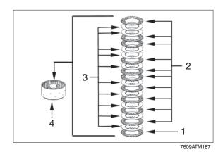
13 Mount end plate (1) and fix disk package by means of snap ring (2) (e.g. thickness = 2.65 mm / recommended value).
