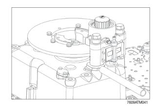
③ Loosen hexagon screws (2) and remove parking brake (1) (see figure TM043).
