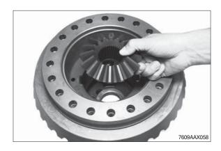
Press crown wheel from the differential carrier.
