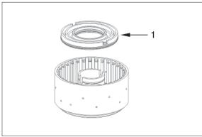
8 Use a hand-operated press to place piston into the disk carrier by means of the assembly aid.
