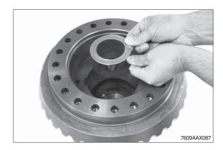
③ Insert axle bevel gear.
