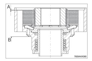
(5) Position housing cover onto pressure piece (see arrow).
