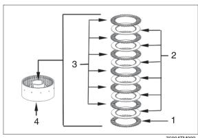
15 Mount end plate (1) and fix disk package by means of snap ring (2) (e.g. thickness = 2.65 mm / recommended value).
