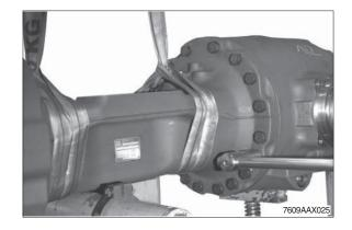
② Loosen the threaded connections and remove the releasing brake tube.
