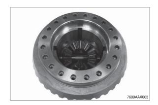
⑤ Remove the second axle bevel gear.
