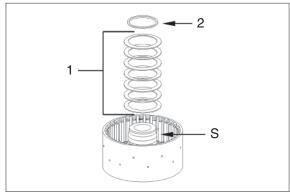
? Preload cup spring package by means of assembly aid (S1) and pressure piece (S2), until L-ring has engaged into the annular groove.
