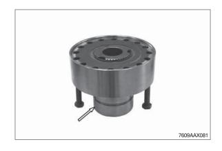
(ii) Position the premounted differential with the lifting device onto the housing cover and preliminarily fix with hexagon screws.
