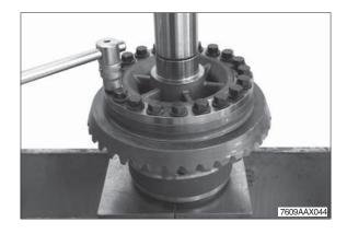
⑦ Remove axle bevel gear with thrust washers from the differential housing.
