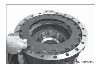
(ii) Loosen hexagon screws, remove releasing cover and cup spring.
