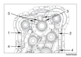
(3) Mount O-rings  $22\times3$  into the annular groove of the oil tubes (1 and 2) and oil them.
