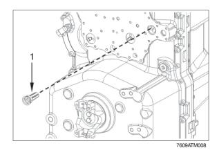
⑥ Mark installation position of wiring harness (1) towards valve block (2).
