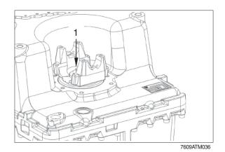
② Pull off output flange (1) and remove shaft seal (2).
