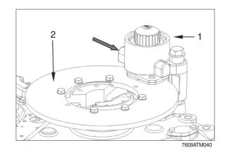
② Loosen hexagon nut with open end wrench insert.
