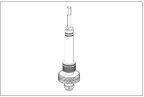
③ Pull tapered roller bearing (inner ring) off the drive gear.
