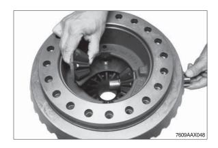
① Remove the axle bevel gear and the shim behind.
