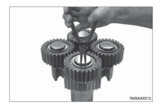
Pull off planetary gear.
