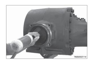
⑤ Insert the determined shim e.g. s = 1.00 mm into the housing hole.
