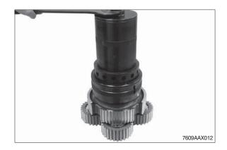
Disengage retaining ring.
