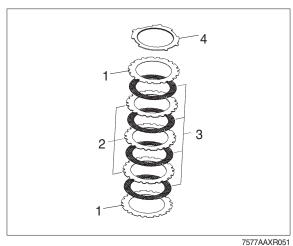
① Insert disc package, considering disc arrangement and installation position of outer discs-see sketch 7577AAXR051.
