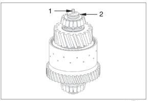
\* Check closing and opening of the clutch by means of compressed air at the hole (see arrow).
