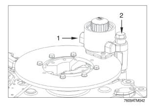
④ Loosen hexagon screws (2) of bolted brake disk/output flange connection and remove brake disk (3).
