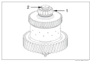
Check closing and opening of the clutch
