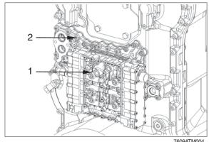
② Remove gear-shift control assy (1) and sealing plate (2).
