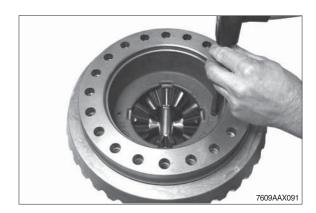
$\ensuremath{{\mbox{$\bigcirc$}}}$  Mount second axle bevel gear.
