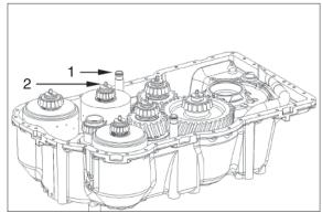
(5) Use lifting device to bring housing rear part (1) into contact position with housing front part (2) again.
