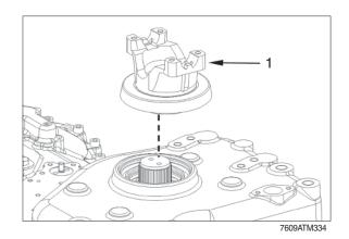
④ Insert O-ring 48×4 into the space between output flange and shaft.
