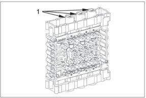
(3) Loosen two Torx screws (1) and preliminarily fix housing by means adjusting screws. (Housing is springloaded) Then loosen remaining Torx screws.
