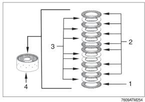
10 Mount end plate (1) and fix disk package by means of snap ring (2) (e.g. thickness = 2.65 mm / recommended value).
