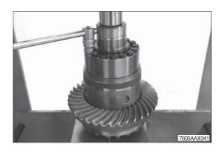
Preload the housing cover/compression spring by means of the press and disengage the retaining ring.
