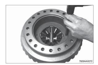
$\ensuremath{{\mbox{$\bigcirc$}}}$  Mount second axle bevel gear.
