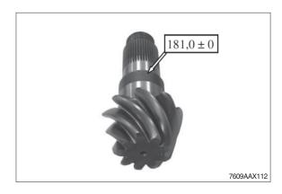
③ Determine dimension III (bearing width).
