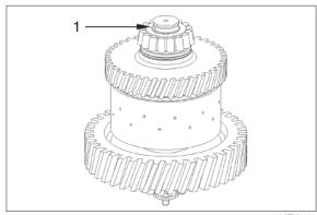
② Pull tapered roller bearing (inner ring) off the shaft.
