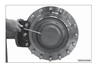
S Loosen locking screws and remove the releasing cover.
