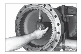
Insert the sun gear shaft until contact is obtained.
