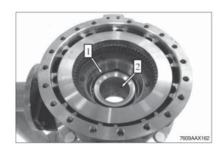
(19) Align disk package centrally and radially.
