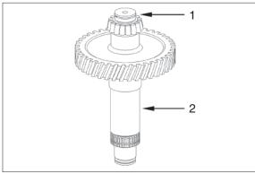
Pull tapered roller bearing (inner ring) off the shaft.
