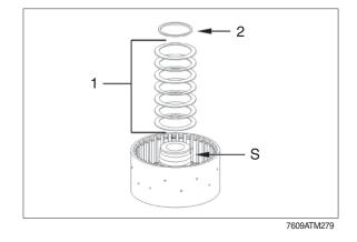
(13) Preload cup spring package by means of assembly aid (S1) and pressure piece (S2), until L-ring has engaged into the annular groove.
