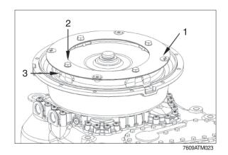
② Separate converter (1) from transmission by means of lifting device.
