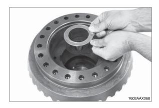
③ Insert axle bevel gear.
