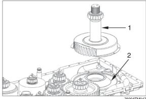
(4) Remove all rectangular rings (1) from the clutches and all O-rings (2) from the oil tubes.
