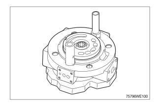
(9) For clockwise rotation pumps the distributor plate is off-set by  $4^{\circ}$  to the right from the centre position.
