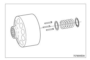
(4) Pre-tension the spring using a suitable device.
