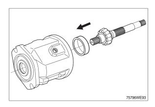
(3) Fit pressure pins using an assembly aid.
