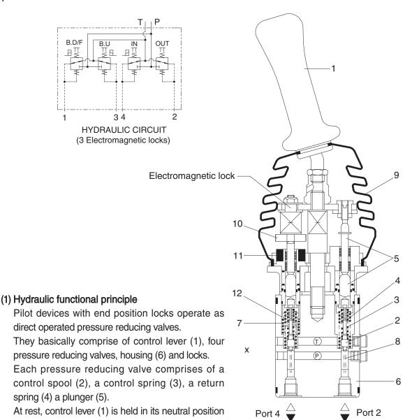
When control lever (1) is deflected, plunger (5) is pressed against return spring (4) and control spring (3).
