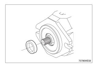
(3) Assemble the sealing ring, fitting tool holds the correct position of the sealing ring in the pump housing.
