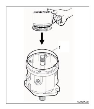
(7) Fit bearing (1) in connection plate.
