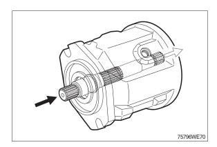
(9) Pre-tension the spring (1) using a suitable device.
