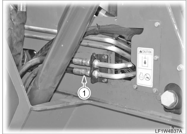
1-3. Disconnect the hydraulic hose (1) to the hydraulic tube from the outside of the right section of the main frame.
