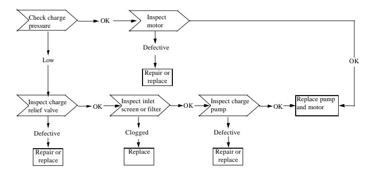
Symptom: System Will Not Operate In Either Direction
