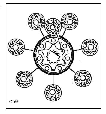
For smooth and continuous motor output rotation, the torque motor utilizes a disc valve which operates in synchronization with the geroler star. The disc valve arrangement consist of a stationary balance plate, rotating disc valve and a stationary valve plate.
