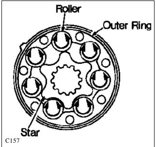
The geroler (fig. C2299), is both a fluid displacement motor and a gear reducer. It provides 8 times (the number of star points) greater power per revolution than a gear, vane or piston type motor. This means that 8 times the greater torque can be developed at one eighth the speed without further gear reduction.
