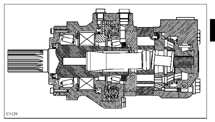
The basic geroter design uses a combination of mechanical and hydraulic principles that are utilized in the high torque, low speed motors.
