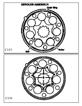
A drive shaft is used to transmit the rotation of the star to the output shaft. The drive shaft has crowned external splines to match the internal splines in the star and output shaft. This type of drive is used because the star center line continuously changes during rotation.
