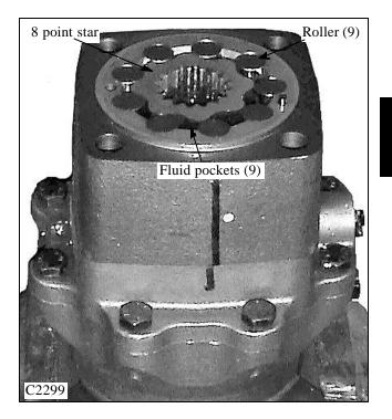
Example shown in fig. C166 is one complete star orbit, or one sixth of the output shaft rotation. The star must travel through 6 complete orbits for each single rotation of the output shaft creating a speed reduction of 6 to 1. The use of 7 fluid power pockets with the 6 to 1 ratio provides 42 fluid power cycles per each complete shaft revolution. **NOTE: Actual star point count is 8. This is only an example.**
