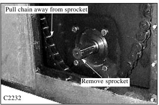
5 Remove the bolt retaining the drive sprocket to the drive motor. (fig. C2272)
