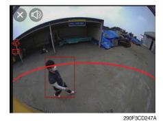
· When a worker/pedestrian reaches the green line, which is an external danger area equipped on the cluster, warning buzzer sounds and it displays a green rectangular box recognizing the worker/pedestrian.
