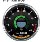
1 This displays the engine speed.
