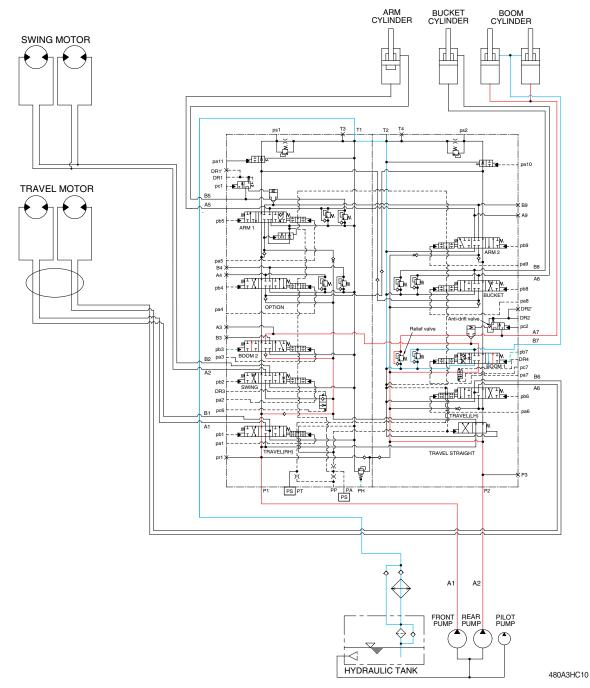
When the RH control lever is pulled back, the boom spools in the main control valve are moved to the up position by the pilot oil pressure (pb3, pb7) from the remote control valve.
