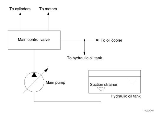
The pumps receive oil from the hydraulic tank through a suction strainer. The discharged oil from the pump flows into the control valve and goes out the tank ports.
