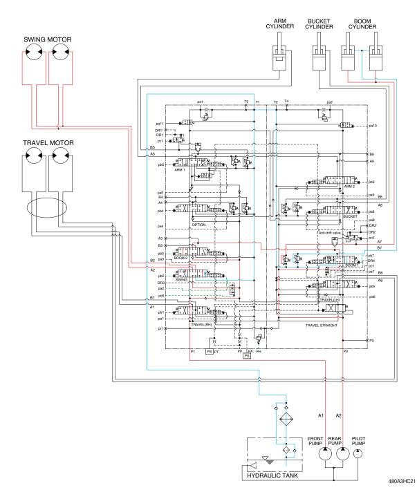
When the swing and boom up functions are operated, simultaneously the swing spool and boom spools in the main control valve are moved to the functional position by the pilot oil pressure (pa2, pb2, pb3, pb7) from the remote control valve.
