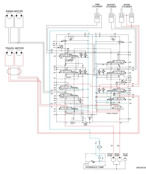
When the boom and travel functions are operated, simultaneously the boom spools and travel spools in the main control valve are moved to the functional position by the pilot oil pressure (pa2, pb2, pb3, pb7, pa1, pb1, pa6, pb6) from the remote control valve and the straight travel spool is pushed to the right by the oil pressure from pilot pump.
