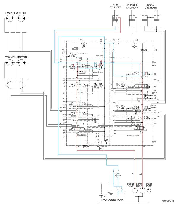
When the LH control lever is pushed forward, the arm spools in the main control valve are moved to the roll out position by the pilot oil pressure (pb5, pb9) from the remote control valve.
