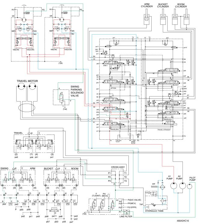
When the LH control lever is pushed left or right, the swing spool in the main control valve is moved to the left or right swing position by the pilot oil pressure (pa2, pb2) from the remote control valve. The oil from the A1 pump flows into the main control valve and then goes to the swing motor. At the same time, the return oil from the swing motor returns to the hydraulic oil tank through the swing spool in the main control valve.
