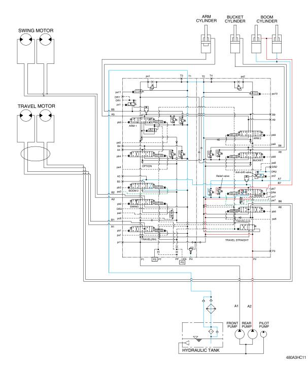
When the RH control lever is pushed forward, the boom spools in the main control valve are moved to the down position by the pilot oil pressure (pa3, pa7) from the remote control valve.
