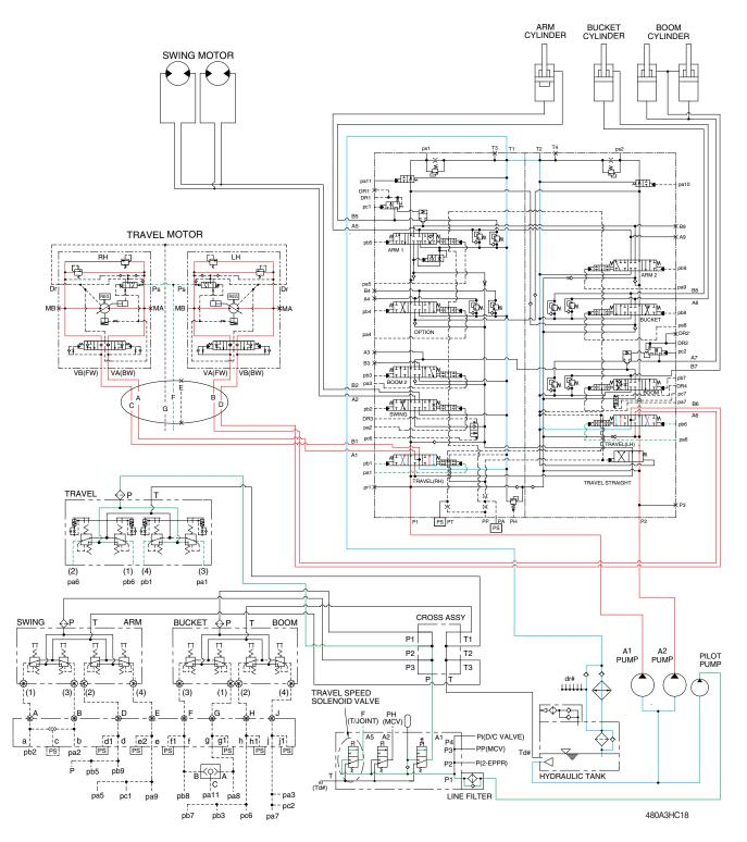
When the travel levers are pushed forward or reverse position, the travel spools in the main control valve are moved to the forward or reverse travel position by the pilot oil pressure (pa1, pb1, pa6, pb6) from the remote control valve.
