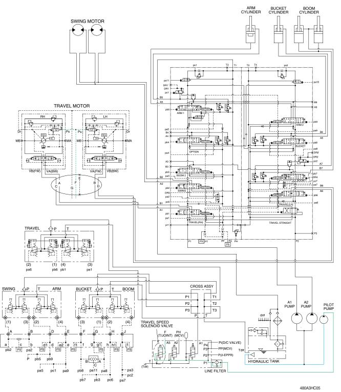
When the travel speed solenoid valve was placed in the Hi position, the pressure oil from pilot pump through line filter flows to port **Ps** of travel speed change over valve, and the control piston is pushed up, thus minimizing the displacement.
