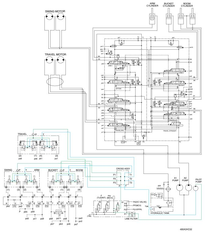
The pilot pump receive oil from the hydraulic tank. The discharged oil from the pilot pump flows to the safety solenoid valve through the line filter. The oil is filtered by the line filter. The pilot relief valve is provided in the pilot pump for limiting the pilot circuit pressure.
