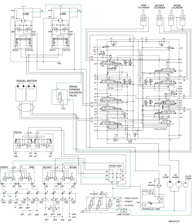
When the swing control lever is tilted, the swing solenoid valve is shifted to the down ward by the MCU that senses the pilot pressure of the swing control lever.
