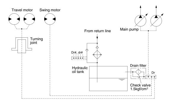
Besides internal leaks from the motors and main pump, the oil for lubrication circulates. These oil have to be fed to the hydraulic tank passing through drain filter.
