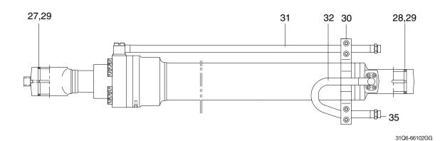
1 Tube assembly 12 Back up ring 27 Pin bushing 2 Rod assembly Cushion ring 28 Pin bushing 13 3 Gland 14 Piston 29 Dust seal 4 DD2 bushing 15 Piston seal 30 Band assembly 5 Snap ring 16 Wear ring 31 Pipe assembly-R 6 Rod seal 17 **Dust ring** 32 Pipe assembly-B 7 Back up ring 18 O-ring 33 O-ring 8 Hexagon socket head bolt Buffer ring 19 Back up ring 34 9 **Dust wiper** 20 Lock nut 35 O-ring 21 10 Snap ring Hexagon socket set screw
