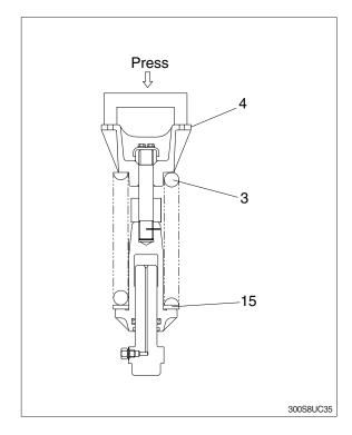
⑤ Lighten the press load and confirm the set length of spring (3).
