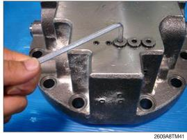
(2) Apply loctite #242 on the NPTF 1/16 plug (2) and then assemble 12-NPTF 1/16 Plug (2) into rear cover(34).
