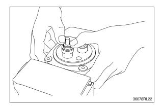
(7) When return spring is strong in force, assemble 4 sets at the same time, utilizing plate (12), and tighten joint (15) temporarily.
