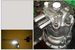
③ Hang valve casing (23) on hoist, unloose socket bolt (37, 38) and disassemble from casing (1).
