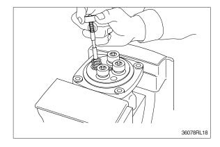
(3) Assemble O-ring (10) onto plug (8).
