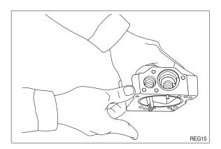
(13) Install cover (C, 629) fitted with adjusting screws (628), adjusting stem (C, 627), lock nut (630), hexagon nut (802) and adjusting screw (924).
