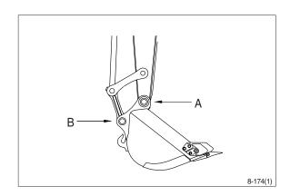
② Remove nut (1), bolt (2) and draw out the pin (A).
