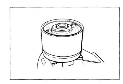
(f) Mount special tool(Special Spanner) to the flange. With the timer spring compressed, remove the washer 5, roller 6 and bushing 7.
