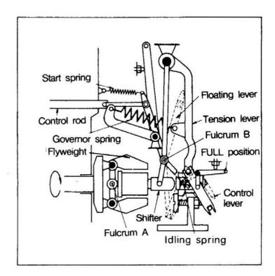
If the load control lever is placed to the idling position after the engine has started, the floating lever will move the control rod back to a position where a fuel injection rate suitable for the idling speed is available, with the point B as the fulcrum.
