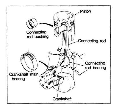
Some of the engine oil which has lubricated the main bearing flows through the oil hole in the crankshaft and lubricates the connecting rod bearing. The oil then flows through the oil hole in the connecting rod and lubricates the connecting rod bushing.
