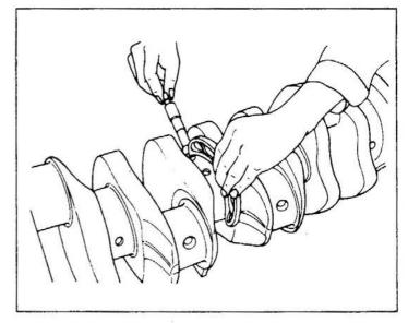
(4) Measure the bend of the crankshaft. If the repair limit is exceeded, correct with a press or grind to undersize.
