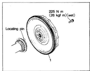
(11) Measure the flywheel mounting condition(runout). If the pointer of the dial indicator deflectis beyond the repair limit, check the bolt tightness or mounting surface.
