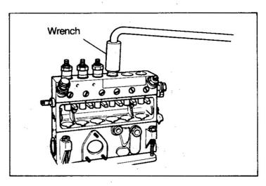
NOTE: Immerse the delivery valve combined with delivery valve seat and the plunger combined with plunger barrel in gas oil without changing their combinations.
