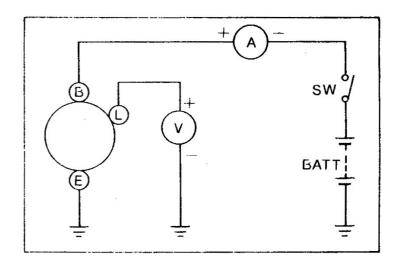
4) Increase the engine speed to approximately 2000rpm and read the regulator voltage value if the charge current is 5A or less.
