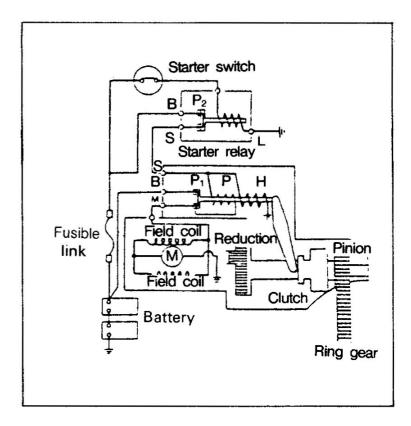
In this condition, no current flows to the pull-in coil.
