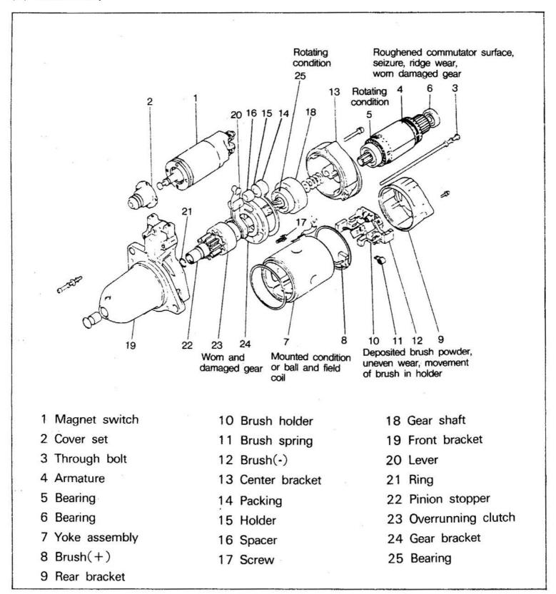
NOTE: 1. Do not remove the bearings located on each end of the armature unless defective.
