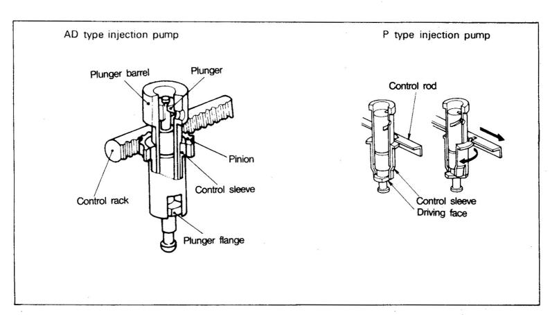
The effective stroke means the length of the plunger stroke from the time when the upper end of plunger closes the inlet-outlet holes of plunger barrel until the oblique groove of plunger opens to the inlet-outlet holes. When the effective stroke stands at zero, it indicates that no fuel injection takes place.
