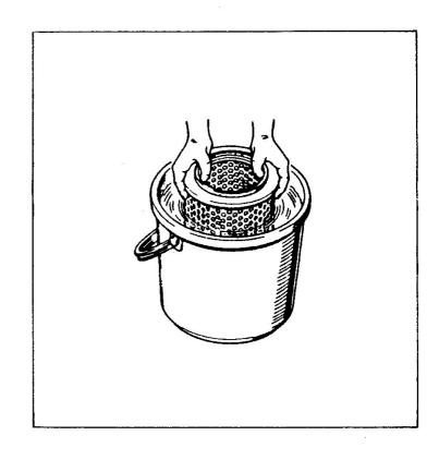
NOTE: When the element has to be quickly dried, an electric fan, etc. may be used, but do not use compressed air or fire.
