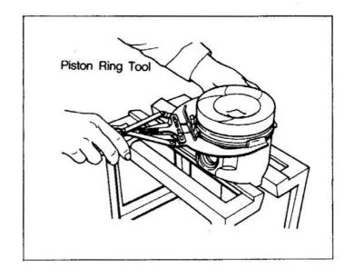
Install the piston ring with the manufacturer's mark at the open end of the ring upward.
