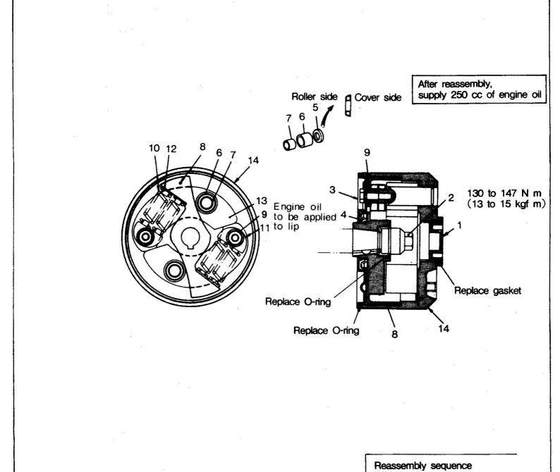
(a) Mount special tool(Base) in a vice and secure the timer housing 14 to the base.
