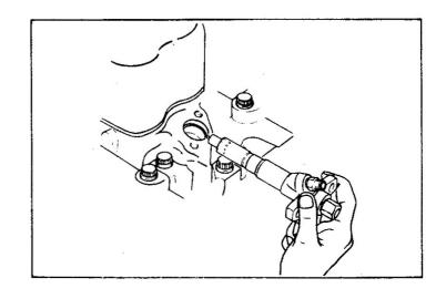
NOTE: Put a cover on the injection nozzle mounting holes and injection pipes to prevent entry of dust and dirt.
