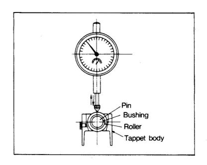
Calculate the clearance between the tappet and pump housing.
