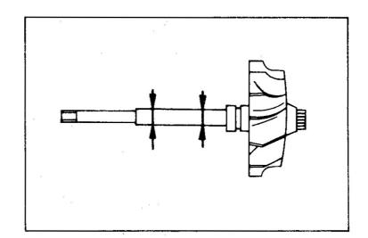
(c) Set a dial indicator beside the threaded portion of the shaft to measure the bend.
