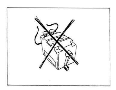
(4) When a steam cleaner is used, take care to prevent direct exposure of the alternator to the steam.
