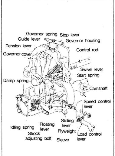
a no-fuel injection state for stopping the engine. A cancel spring is provided to make sure that when the lever is operated, no undue force is applied to the link.
