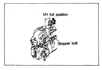
Slowly increase the pump speed from Nc and press down the adjusting lever and adjust the maximum speed stopper so that when the speed reaches Nd, the control rack will begin to retreat from the position Rc.
