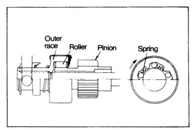
When the armature turns, the rotation is transmitted through the rollers to the pinion by the wedge action of the outer race of the clutch.
