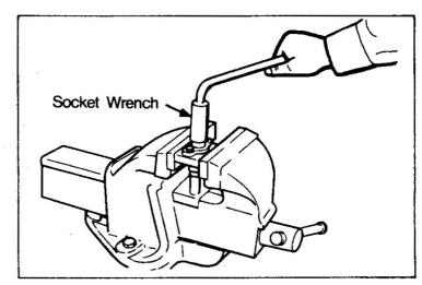
(q) Remove the governor side screw bushing 29 with special tool (Special Wrench) and remove the pin 30 and bushing 31.
