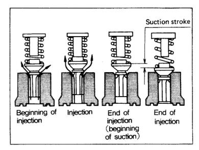
The delivery valve is further brought down until it is held against the seat surface tightly. The amount of fuel corresponding to the stroke during the period is drawn back from above to instantly lower the residual pressure in the line between the delivery valve and nozzle. The draw-back effect improves the cutting of fuel from the nozzle and prevents after-injection dripping.
