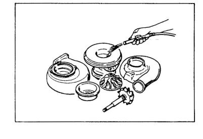
(f) To prevent rust, apply engine oil to the entire internal and external surfaces of the bearing housing, turbine housing and turbine backing plate and the shaft portion of the turbine wheel shaft.
