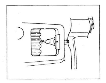
Crank the engine another rotation and check and adjust the valve clearance of all the valves.
