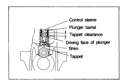
4) If the tappet clearance is less than the nominal value, adjust within the extent permitted by the injection start interval.
