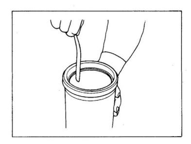
(5) Calculate the clearance from the piston pin O.D. and piston I.D.
