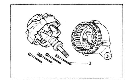
(b) Unsolder the stator coil leads and remove the stator 10 from the rear bracket 9.
