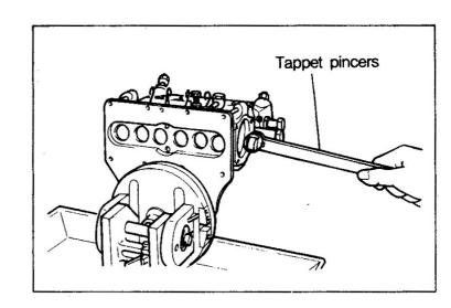
(f) Push the tappet inserted into the housing up with special tool(Roller Pincers) and insert special tool(Tappet Pin) into the hole in the tappet.
