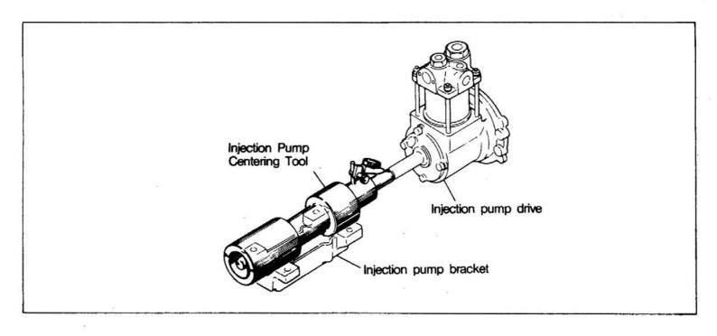
2) Slide the dial indicator of the centering tool toward the injection pump drive and measure the positions of the injection pump drive shaft shown in the illustration with the dial indicator.
