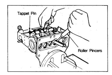
(k) Hold a tappet in special tool(Tappet Pincers), remove the special tool(Roller Pincers), and then take out the tappet 9 and shim 10.
