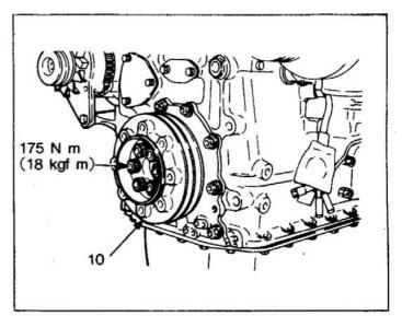
7-3-2 Flywheel, Timing Gear and Camshaft
