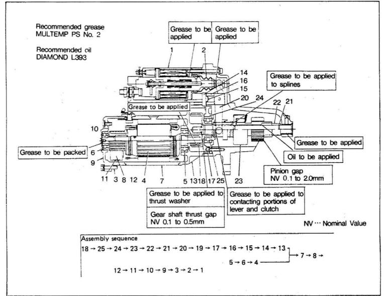
NOTE: 1. When the lever is installed, pay attention to its installing direction.
