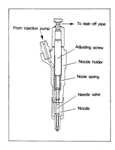
The injection pressure of the injection nozzle is adjusted by changing the tension of the nozzle spring with the adjusting screw.
