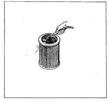
NOTE: Do not strike the element or strike it against a hard object to loosen the dust.
