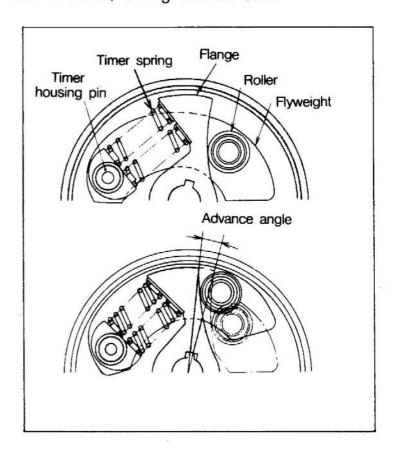
In this manner, the roller installed on the flyweight moves the flange in the turning direction and advances the injection timing.
