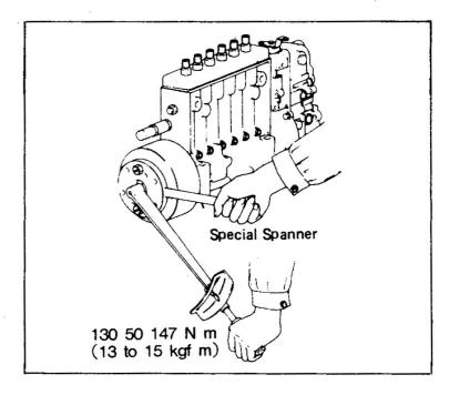
(d) Remove the plug at the rear end of the timer and supply 250 cc of engine oil.
