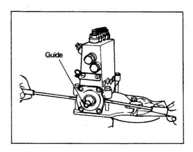
(j) Push the tappets up from the bottom of the injection pump with special tool(Roller Pincers) and remove the special tools(Tappet Pins).
