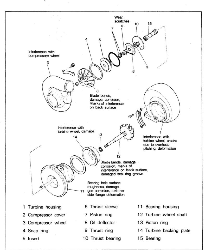
(1) Hold the flange portion of the turbine housing in a vice.
