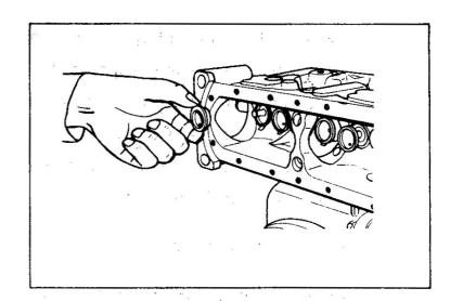
(I) Remove the plunger 13, using special tool(Plunger Insert).
