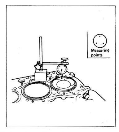
NOTE: Make sure that the piston projection is up to specification, because an incorrect projection could cause adverse effects on engine performance.
