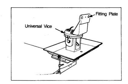
(b) Remove the pipe joint bolt and overflow valve from the fuel inlet of the injection pump. Utilizing the threaded hole, install special tool(Plate).
