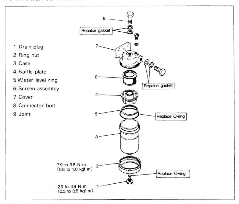
If the red float in the translucent case rises to the level of the red line marked on the outer circumference of the case, immediately loosen the drain plug to discharge water. It is not necessary to completely remove the drain plug, as water is discharged gradually through the groove of the looaened plug.
