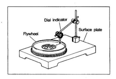
NOTE: If the ring gear shows an abnormal condition, replace the ring gear before measurement. (3) If the distortion of the surface making friction with the clutch is in excess of the repair limit, grind.
