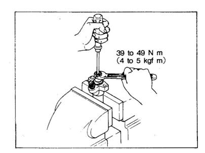
5) After the cap nut has been tightened, recheck whether the injection pressure is correct.
