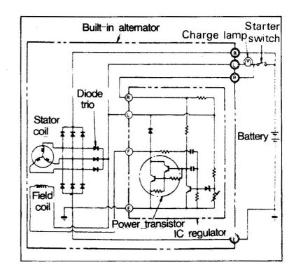
3. To make sure that the voltage builds up easily, power transistor base current is kept flowing. Therefore, when the battery switch is in closed position, current(10 mA or less) continues to flow through the regulator even when the engine is stationary.
