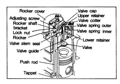
(a) Both inlet and exhaust valves are made of surface-treated heat-resisting steel. The valve seat angle is 45°.
