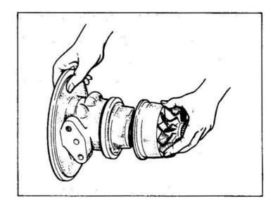
NOTE: 1. There are two pins driven into the turbine housing. Do not remove the pins.
