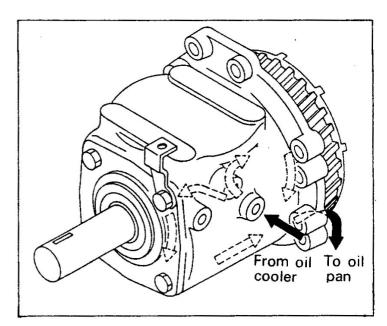
For lubrication of the parts, the engine oil is drawn by an oil pipe from the engine oil cooler. The oil flows through the oil hole in the shaft and lubricates the bearing.
