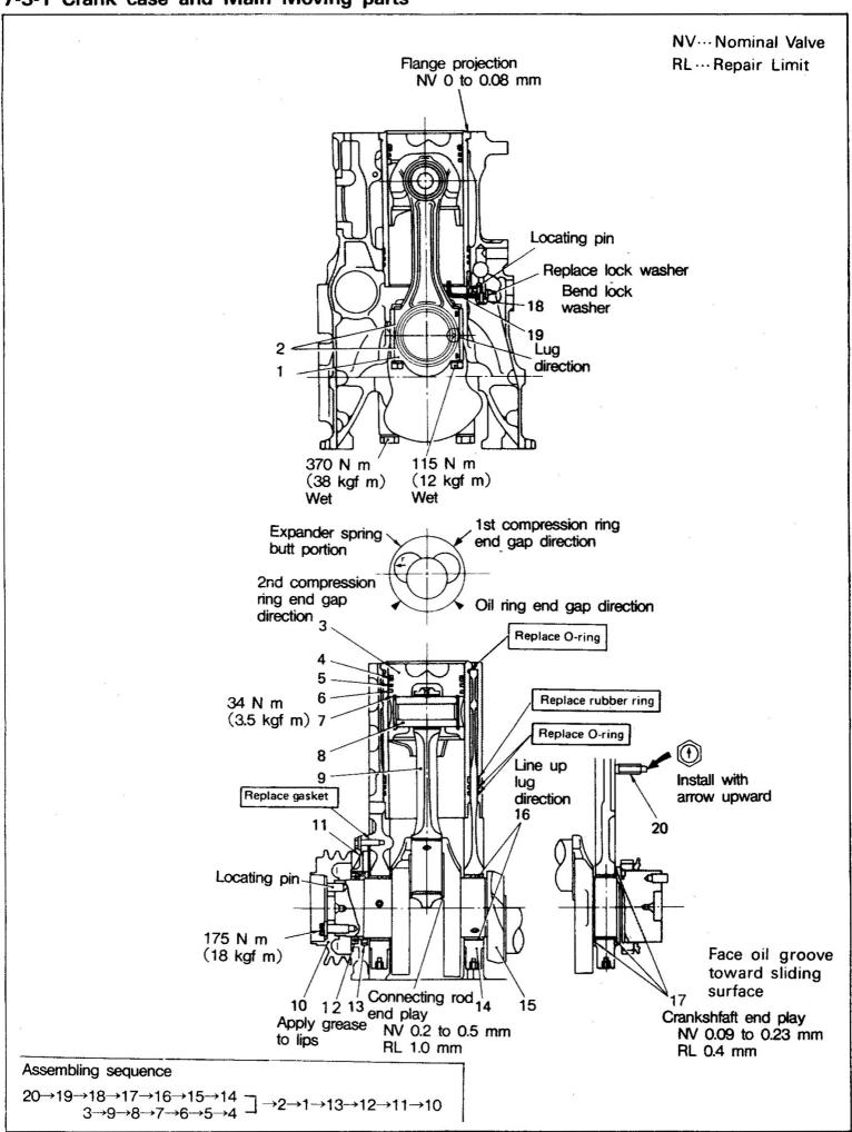
Install the oil spray plug 20 to the crankcase.
