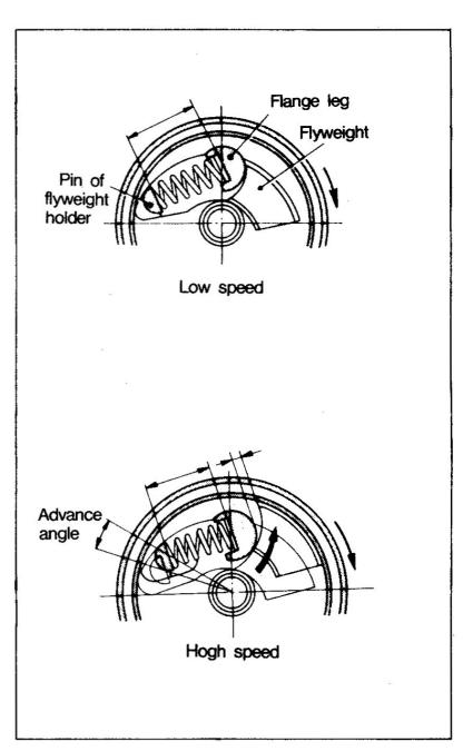
If the engine speed changes from a high to low speed, the centrifugal force of the flyweights will decrease and the flyweights will return to their original positions. At the same time, the pins of the flyweight holder will be pushed back by the timer springs.
