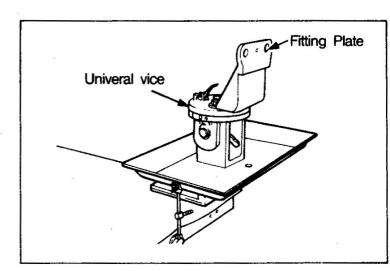
(c) Remove the pipe joint bolt 1 and overflow valve 2 from the fuel inlet of the injection pump. Utilizing the threaded hole, install special tool (Plate).
