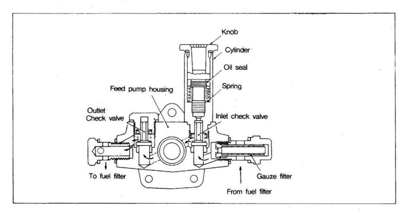
The feed pump feeds fuel under pressure as follows.
