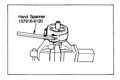
(i) Inject approx. 150g of automatic timer grease from the timer plug hole.
