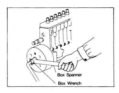
(c) Mount special tool(Special Spanner) by taking advantage of the coupling mounting thread. While holding it to prevent turning, remove the timer from the injection pump, using special tool(Extractor).
