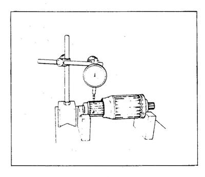
b) Measure the outside diameter of the commutator. If the outside diameter is less than the service limit, replace the armature.
