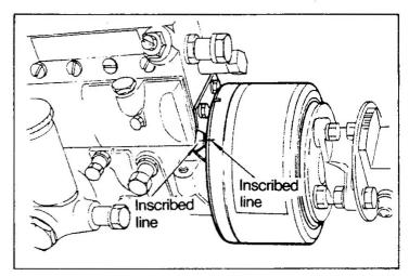
4) Install the driving coupling together with the coupling plate on the injection pump drive shaft.
