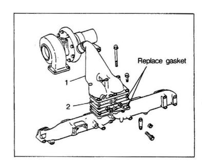
NOTE: When the air heater is installed, make sure that the embossed arrow mark of the air heater is directed toward the inlet manifold.
