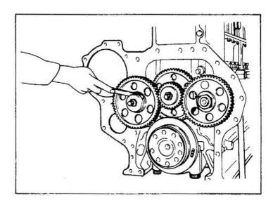
(5) Loosen the thrust plate mounting bolt through the camshaft gear hole and remove the camshaft 6.
