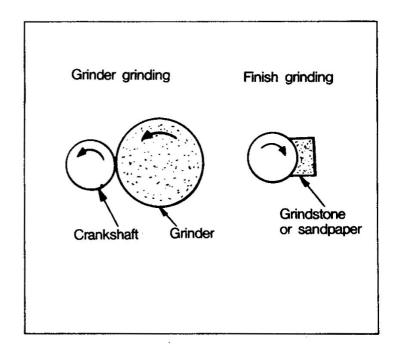
(f) To finish the crankshaft with a grindstone or sandpaper, turn the crankshaft counterclockwise.
