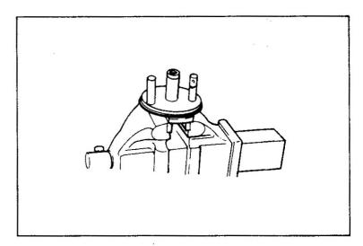
(e) After placing special tool(Support) on the flyweight, install the shim 8 and spring 7.
