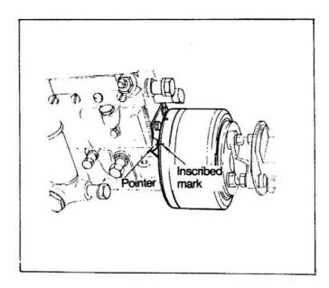
(3) If the fuel injection start timing is not correct, loosen the two timing adjusting bolts and adjust the timing by turning the automatic timer.
