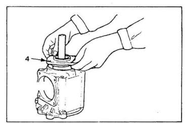
(3) Remove the shaft 6 from the crankcase 9.
