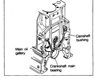
(c) The engine oil that has lubricated the No. 7 camshaft bushing is routed through the oil holes in the top of the crankcase to each cylinder head.
