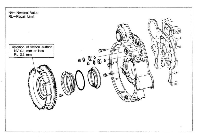
BD···Basic Diameter NV···Nominal Value RL···Repair Limit SL···Service Limit
