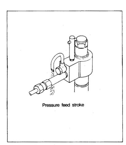
5) Slowly turn the camshaft until the fuel ceases to flow from the overflow pipe of the nozzle holder (until static injection begins).
