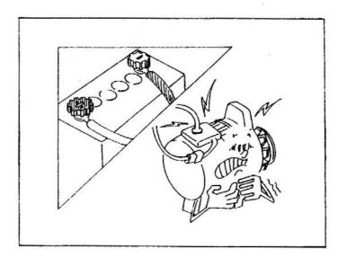
(2) Do not disconnect the battery terminal connections while the engine is running. Otherwise, a sure voltage will be generated, causing deterioration of the diode and the regulator.
