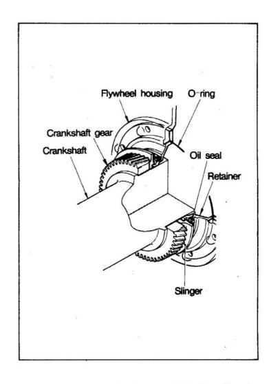
The front portion of the crankshaft is a flange type to which the crankshaft pulley is mounted with bolts. A torsional damper mounted to the pulley absorbs the torsional vibration of the crankshaft.
