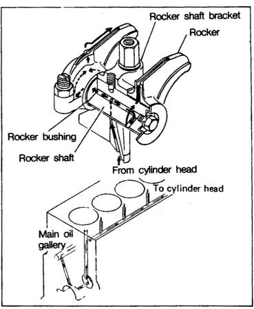
ting screw portion, flows through the cylinder head and crankcase push rod hole, lubricates the tappet and camshaft cam portion, and returns to the oil pan.
