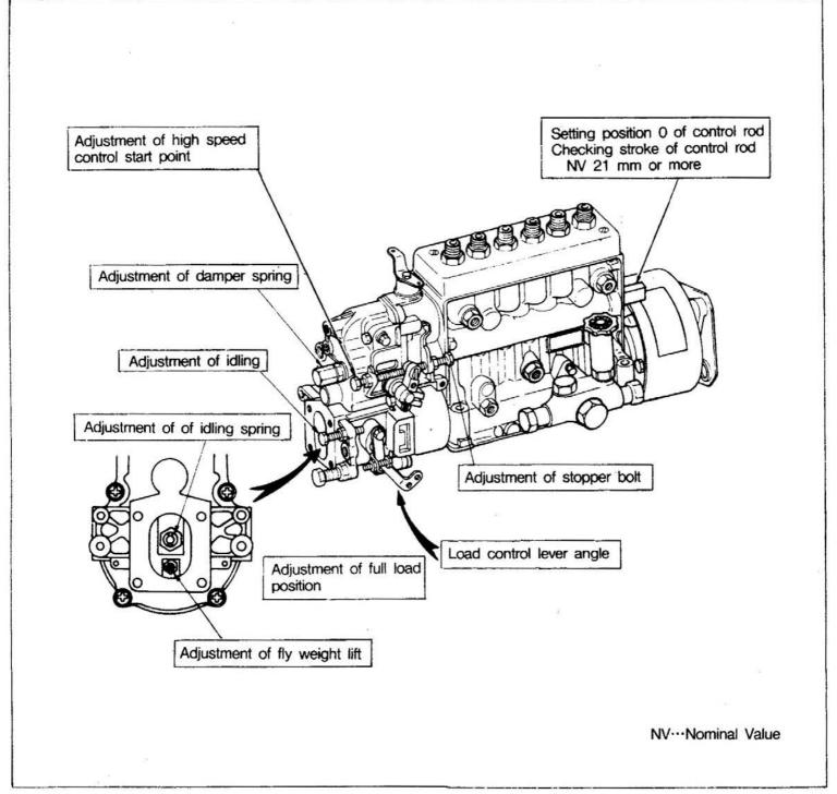
NOTE: 1. Remove the damper spring.
