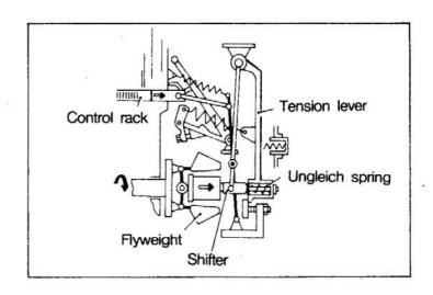
As the engine speed increases, the centrifugal force of flyweight increases. If it becomes larger than the pressure of the Ungleich spring, the Ungleich spring is slowly compressed before the start of high speed control, and the control rack moves in the direction that fuel is reduced. The Ungleich stroke is completed at the position where the control block directly touches the tension lever.
