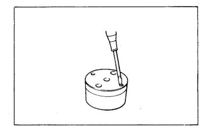
(f) Using special tool(Hand Spanner), remove the timer case 3 by turning clockwise.
