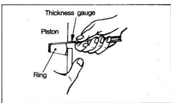
(4) Place the piston ring in a standard gauge or new cylinder to measure the open end clearance.
