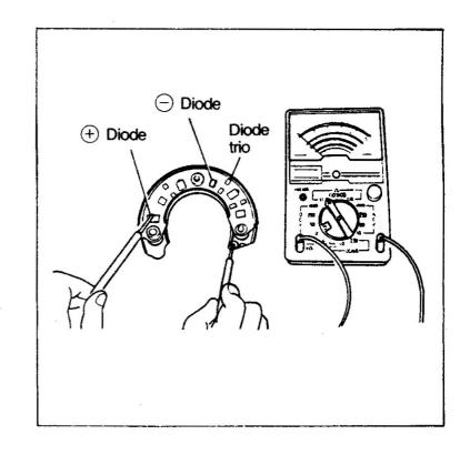
Replace the rectifier if the diode is open or shorted.
