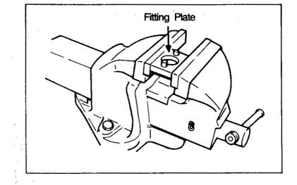
(p) Secure the plunger lock assembly to the special tool(Fitting Plate) and loosen the delivery valve holder with special tool(Socket Wrench).
