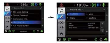
$\cdot\,$  This can confirm the identification of the cluster, MCU, engine and machine.
