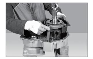
(19) Remove the internal baffle plate (32).
