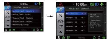
$\cdot\,$  The active faults of the MCU can be checked by this menu.
