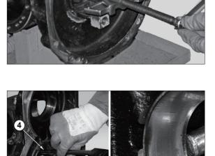
Remove the thrust block of the internal bearing (4) as well as the shim washers (10) (S).
