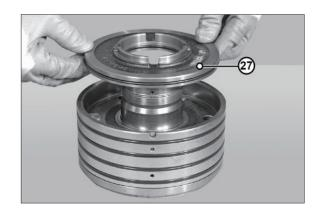
(I) Insert at the bottom the piston of the negative brake (27) and screw up the slotted nut (29).
