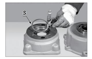
(10) Apply loctite 510 to the machined surfaces.
