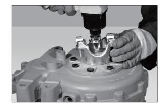
(7) Remove the nut (1) and O-ring (2) and pull out the flange (3).
