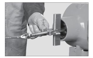
1 Insert a drift in the appropriate holes.
