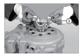
(45) Lubricate the O-ring (2) with grease and fit in the flange (3) seating.Spread with loctite 242 the lock nut (1) and fit.
