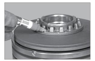
Is Bring the piston group below a press, compress the cup springs and loosen the metal ring.
