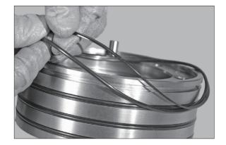
③ Insert the service brake piston (4) hammering alternately with a plastic hammer.
