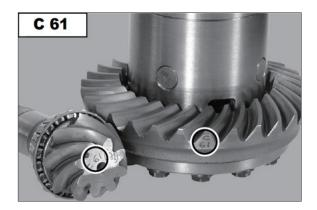
⑤ Calculate shims "S" for insertion under the thrust block of the inner bearing using the following formula :
