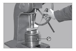
③ Screw down the slotted nut to the earlier determined position.
