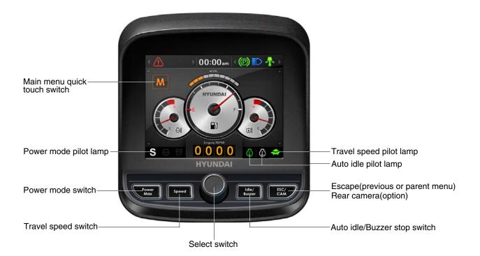
When the switches are selected, the pilot lamps are displayed on the LCD. Refer to the page 4-11 for details.
