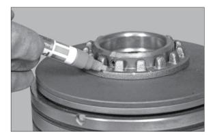
(5) Bring the piston group below a press, compress the cup springs and loosen the metal ring.
