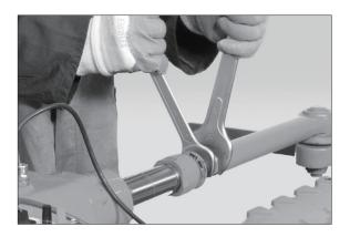
2 Hold the articulations still and rotate the 240 - 270 Nm Loctite 242 Once the convergency has been 24.5~27.5 kgf · m (177~199 lbf · ft)
