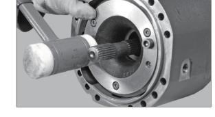
Insert the negative brake unlocking screw (30) up to the end stop.
