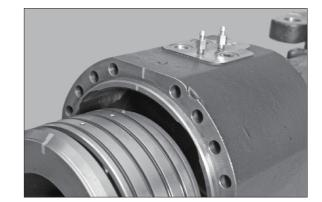
Insert the piston to the end stop by alternating light strokes and remove the screws.
