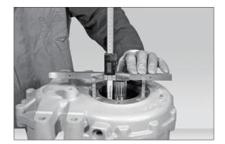
(35) Calculate thickness "S3" of the shims by using this formula : S3 = C - X = S3, where X is the predefined axial backlash.  $X = backlash = 0.15 \pm 0.35$  mm Example : S3 = C-X = 0.45 - 0.25 = 0.20 mm = S3
