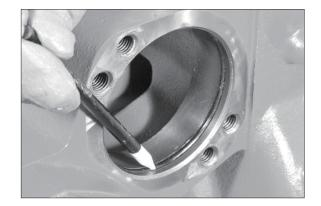
Check that the O-rings (17) (15) of the axle unit are in good condition ; lubricate the seats of the seals and fit the steering cylinder (3).
