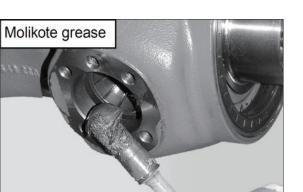
Fit the unit (20) in the steering case (14).
