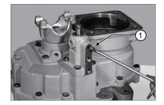
(3) Use a magnet to remove the spring (2) from the gear selector.
