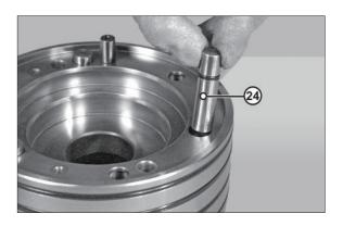
② Remove the O-rings and the anti-extrusions rings from the service brake, the negative brake piston and from the piston.
