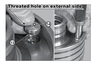
Apply loctite 242 to the thread of the adjustment screw.
