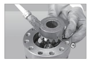
$\circledast$  Insert planetary gear wheel (16).
