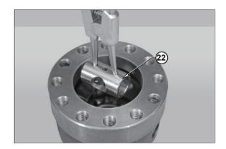
② Remove the planetary gear (16).
