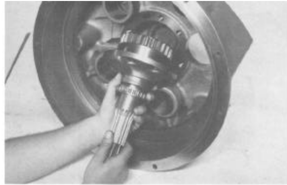
Figure 32 Remove support and turbine shaft assembly. NOTE: If converter housing has a bore plug in the rear center line, remove plug. Remove turbine shaft gear retainer ring. Remove support and turbine shaft assembly. Turbine shaft gear will remain in rear of housing. This is a special ratio gear and is larger than the support bore.
