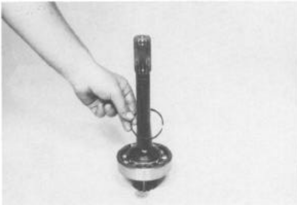
Figure 36 Remove turbine shaft oil sealing ring.
