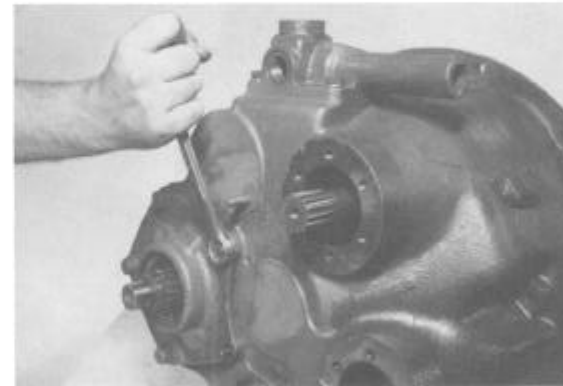
Figure 28 Remove output shaft bearing retainer bolts, stud nuts and washers.
