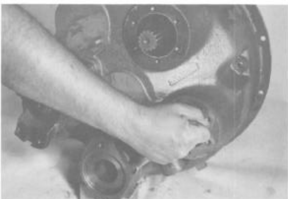
Figure 19 Remove accessory pump drive adaptor bolts.
