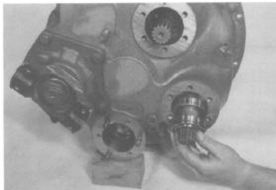
Figure 25 From rear of housing remove pump drive shaft and bearing assembly.
