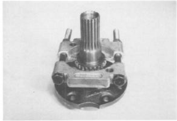
Figure 38 If support bearing is to be removed procedure shown with split puller is recommended.
