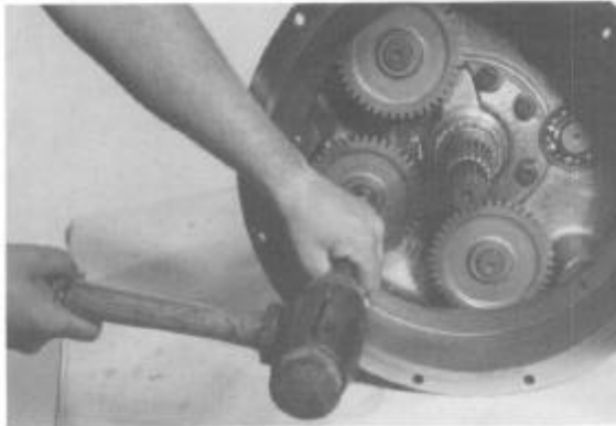
Figure 24 Tap on pump shaft. Remove pump drive gear.
