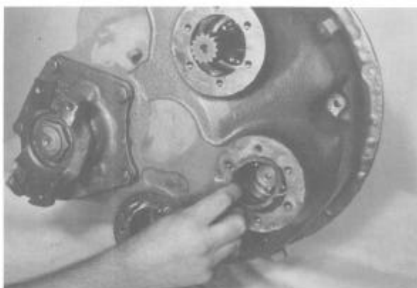
Figure 22 Remove pump shaft retaining washer.
