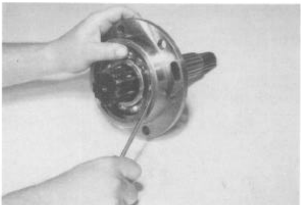
Figure 34 Remove turbine shaft bearing retainer ring from support.
