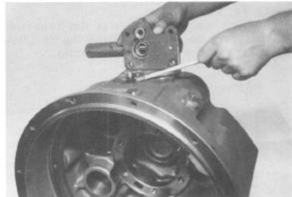
Figure 40 Remove pressure regulating valve, safety valve plunger and spring.
