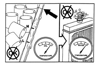
Overfilling with oil raises the oil temperature which is transferred to the coolant system at the oil cooler.
