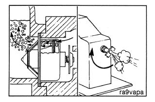
NOTE: A 50 percent mixture of antifreeze and water must be premixed before filling the system. The ability of antifreeze to remove heat from the engine is not as good as water, so pouring antifreeze into the engine first could contribute to an over heated condition before the liquids are completely mixed.
