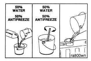
Caution: Never use water alone for coolant. Damage from corrosion can be the result of using water alone for coolant. The small holes in the head gasket are especially susceptible to plugging. These holes are orifices and their size is critical. Do not enlarge the size of the orifices. To do so will disturb the coolant flow and will not solve an overheating problem.
