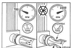
A worn or malfunctioning water pump will not produce the flow required to prevent the engine from running hot. However, be sure to check the other possibilities indicated in the Troubleshooting Logic before checking the flow or replacing the pump.
