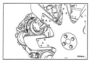
The coolant flow can also be reduced if the inlet hose to the water pump collapses. A hose will usually not collapse while the engine is running at low speed. Check the hose while the engine is running at rated speed.
