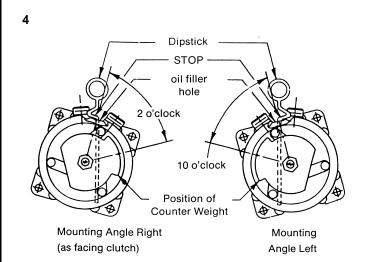
Determine if the compressor is an "angle right" or "angle left" mounting. See illustration. Turn the compressor clutch plate hex nut with a wrench to the 2 o'clock position for angle right mounting, or to the 10 o'clock position for an angle left mounting.
