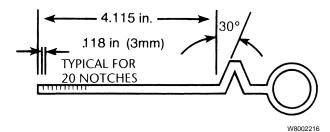
**Note:** If tool J43338 is not available, an oil dipstick can be fabricated from a welding rod, coat hanger, etc., using these specifications.
