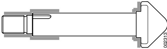
Area for checking for cracks on lift shoe.
