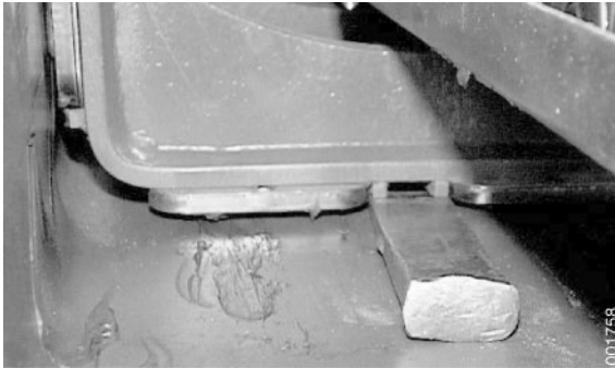
The illustration shows the inner slide plates in the attachment's main beam.
