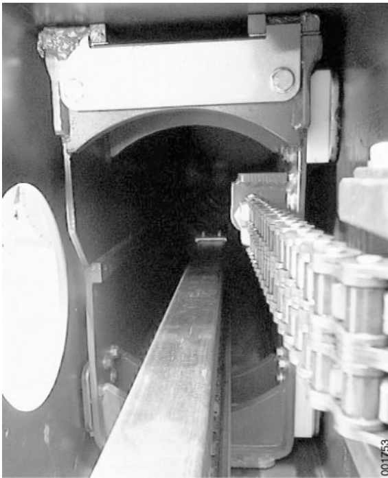
The illustration shows the inner slide plates in the attachment's main beam.
