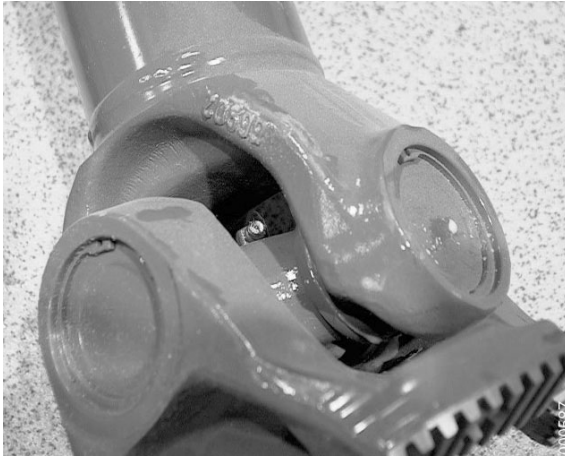
Grease nipple for universal joint, example
